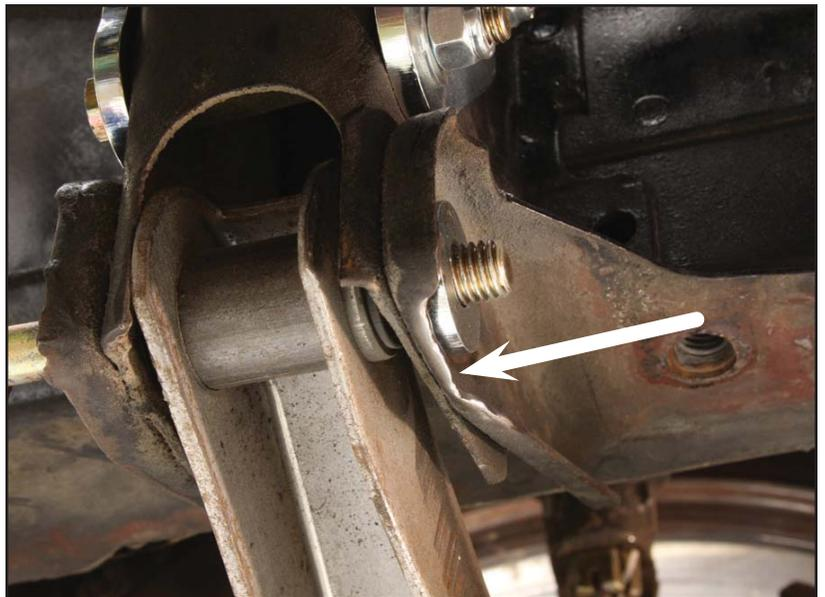
20. Bolt the lower rack brackets to the lower control arm mounts using the orientation and hardware shown on page two. The bracket's bend will face inward or outward depending upon the year of the vehicle.
