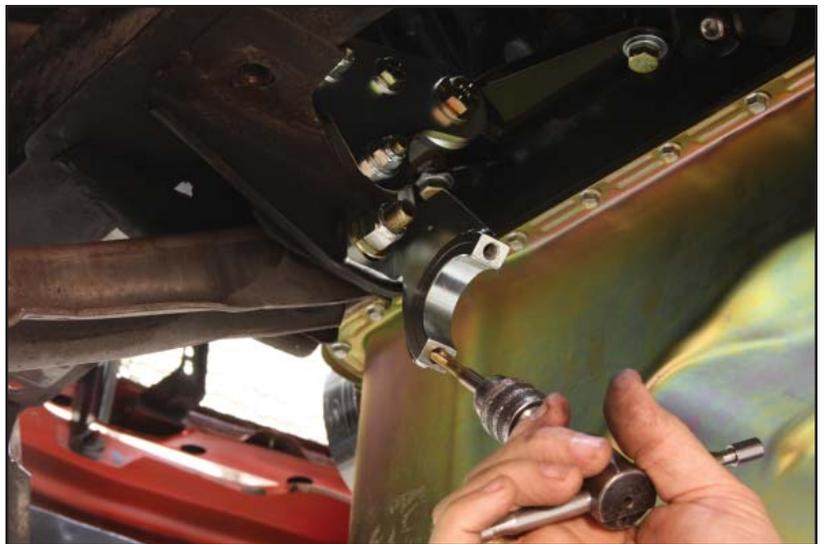
24. Using a 1/2-13 tap, chase the threads of the factory-crossmember mounting holes.
