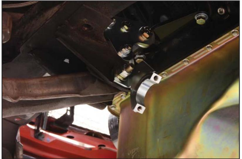
23. Using a 5/16-24 tap, chase the threads of the split collar brackets.
