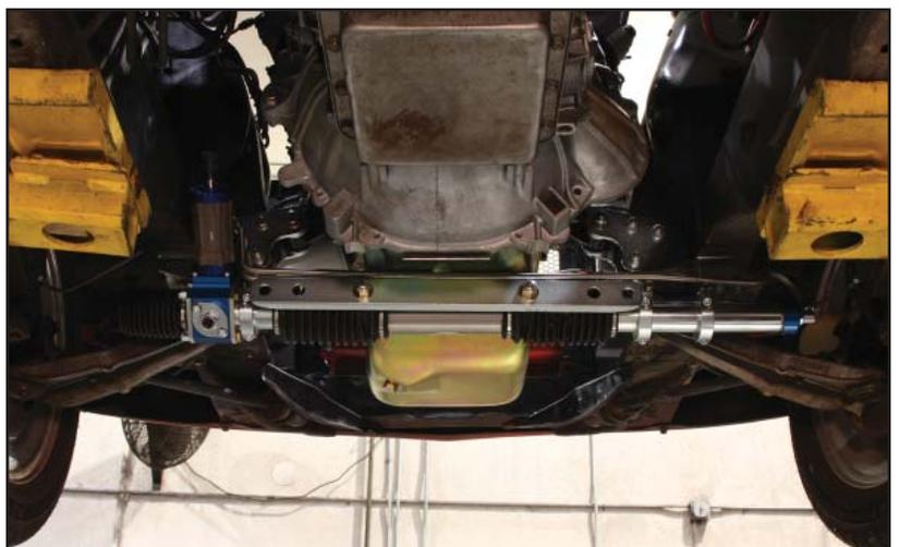
34. Verify that each of the three clamps are just tight enough to correctly align the bracket with the rack tube before lightly tightening the outer-bracket bolts into the frame rails.
