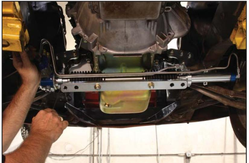
27. On driver-side frame rail, loosely bolt the rack and pinion's attached frame bracket to the OEM-crossmember mounting point, using the same hardware as the passenger side bracket.
