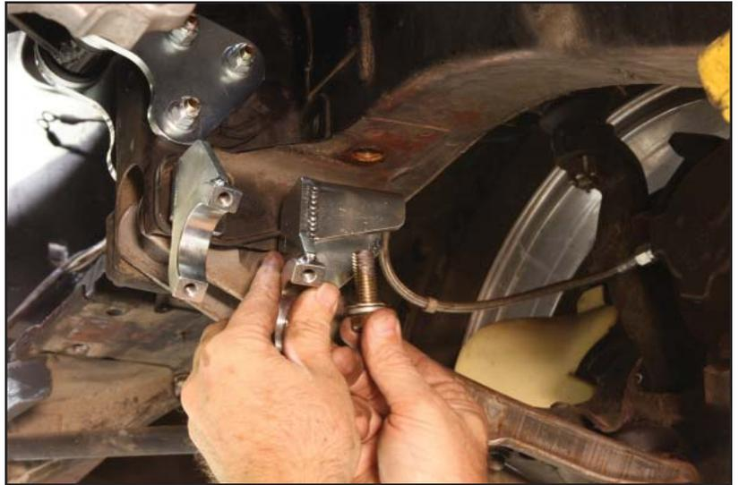
26. Raise the rack-and-pinion assembly into position along the loosely installed brackets.
