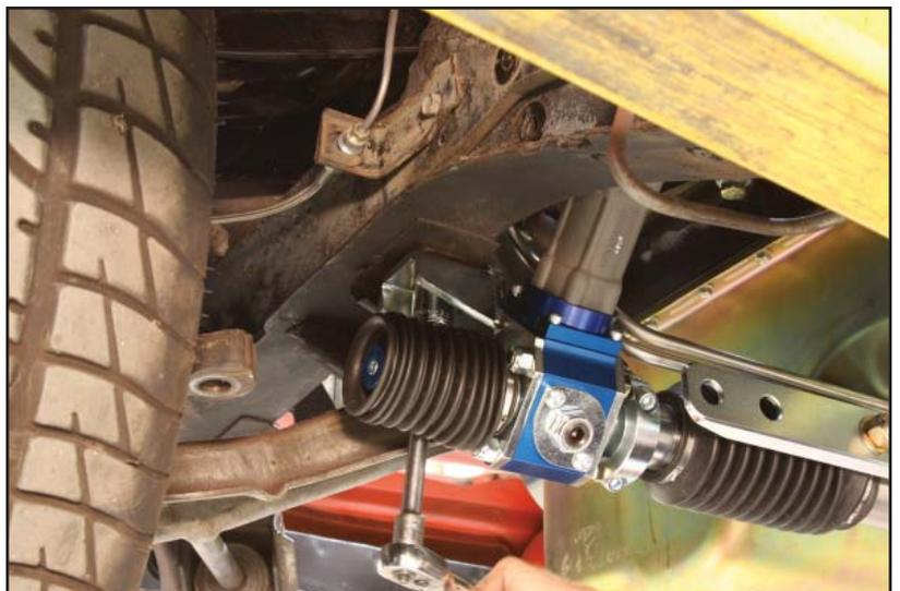
28. Loosely install each of the clamp collars (Item 2) onto their respective brackets so that the clamps seat against the rack tube to prevent rocking, but still allow rotation and sliding movement. A light lubricant can be used to more easily permit sliding of the brackets.
