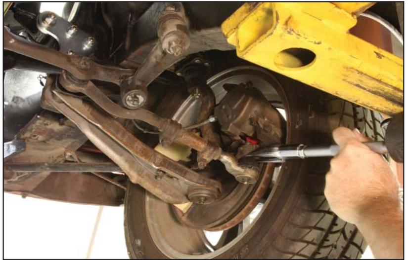
9. Remove the tie rods using a balljoint separator or similar tool.
