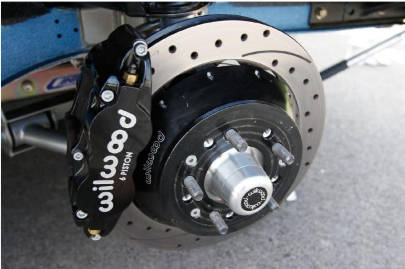
**Wilwood 6-six-piston calipers provide more than enough braking power for the Mustang. They are nicely modulated and look very racy.**
