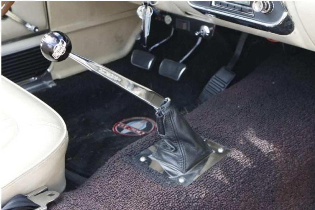
**The Hurst handle is connected to a smooth-shifting Tremec six-speed.**
