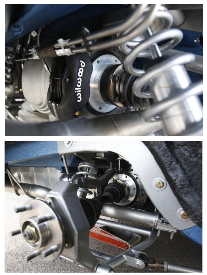
Inboard rear brakes reduce weight at the wheel, which helps cornering performance and ride quality.
