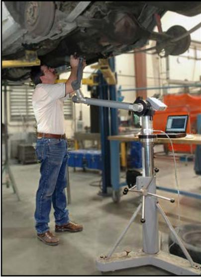
precise three-dimensional digitization of vehicle surfaces and mounting points, accurate to within .003". To begin, multiple identical vehicles are extensively measured to find the OEM tolerance range we must accommodate in our final design. From these scans, an exact model of the vehicle chassis is created in our Pro/ENGINEER software. Engineers can then accurately and efficiently design systems, simulate movement or conditions,
