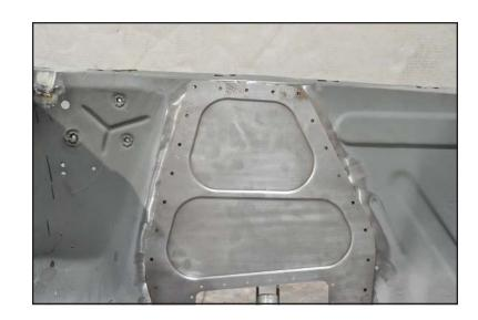
46. When viewed from the outside, spacing between the bead-rolled edges and the opening is not critical. Splash flap alignment and the top edge alignment determine the correct position.
