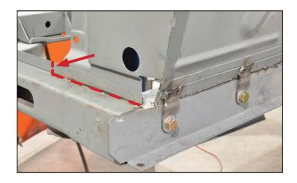
21. From the outside, cut away the flange that spans the shock tower opening.
