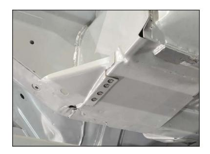
3. With spot welds drilled the gusset can be cleanly removed.
