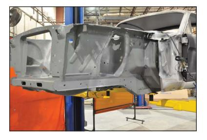
If the vehicle has torque boxes installed, the triangular gusset must be removed by drilling out the spot welds. A replacement gusset is provided. The torque box structure can remain in place during the rest of the installation.
