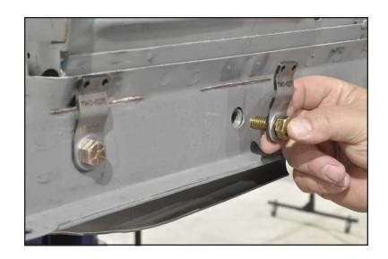
7. Securely tack weld the alignment tabs to the inner fender. These tabs are used to locate the replacement subframe later on.
