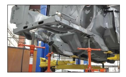
24. Make the vertical cuts on the outside and inside of the frame rail. Do not cut through the bottom part of the rail at this time.
