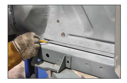
16. The core support crossmember is cut from the front side.
