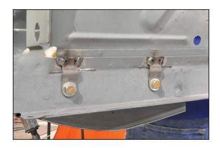
8. Measurements for the next few steps are taken from the inside surface of the lower control arm mounts.
