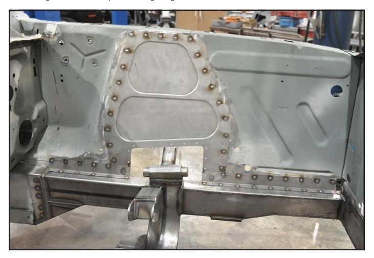
48. Rear Weld Flange - Front edge is flush with splash flap opening. Rear edge is notched for tighter fit over factory rail.
