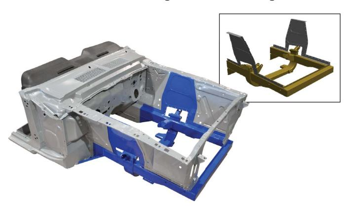
**Description:** Weld-in front subframe clip system replaces factory frame rails, lower radiator core crossmember and shock towers.
