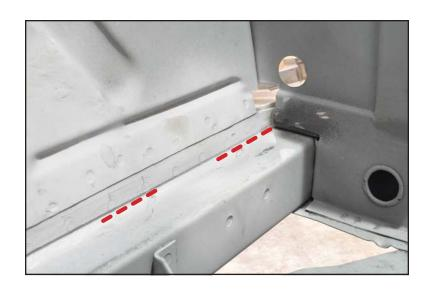
6. Bolt the alignment tabs to the bumper mounting holes.
