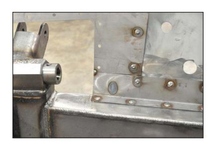
50. Beginning at the joints between the delete panel and weld flanges, plug weld each of the rosette holes before fully welding the seam.
