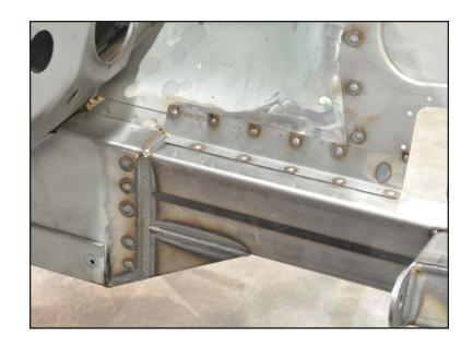
49. Forward Weld Flange - Rear edge is flush with splash flap opening. Front edge is trimmed at core support if needed.
