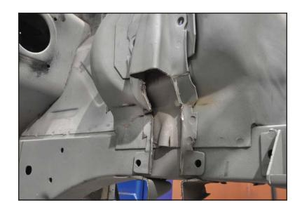
19. Make sure to avoid cutting through the alignment tabs when finishing the cut along the forward length of the inner fender.
