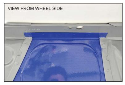
43. On the engine bay side, use a scotch brite pad to clean 1" around the shock tower opening down to bare metal.
