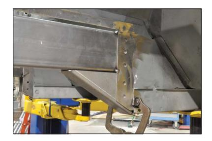
36. Weld the rosette holes before fully welding all seams.
