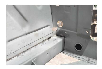
20. Make the final cuts along the front of the core support. The vertical cut is left a little long, but can be trimmed to match the radiator opening once the subframe has been removed.
