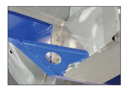
57. Frame Gusset (without torque box) - A small bit of trimming is required along the gusset edge that meets the outrigger closest to the frame rail.
