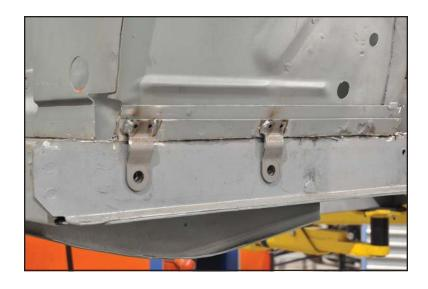
26. Make the final cut through the bottom of the frame rail.
