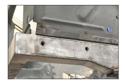
60. Welding portion of the installation is complete.
