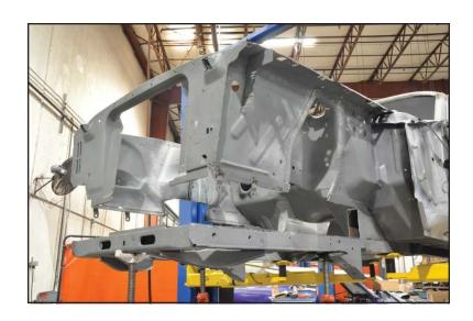
28. Drill three 3/8" rosette holes, 1" in from the edge, and at 3/4", 2", and 3-1/4" down from the top edge of the frame rail. This is repeated for the inside and outside walls of each frame rail.
