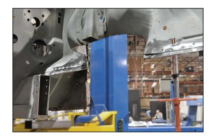
30. Raise the new subframe assembly into position. Factory frame rail position will vary between vehicles and minor working of the factory rail may be required.
