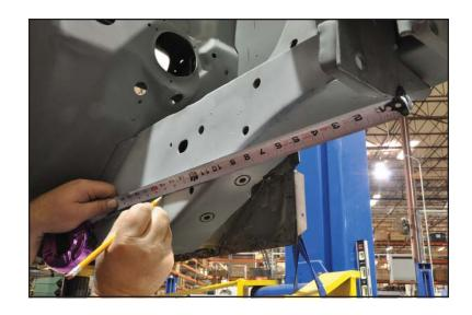
10. Use a square to extend the line perpendicular to the top of the frame rail.
