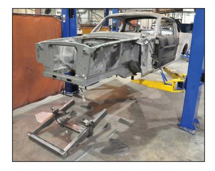
The replacement subframe ships as a factorywelded assembly. Additional accessories include shock tower delete panels, inner fender weld flanges, and under rail gussets.
