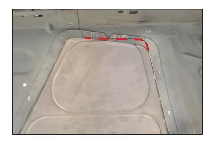
47. Fitment of the delete panel and forward and rear weld flanges, that tie the inner fenders to the frame rail, needs to be done simultaneously.
