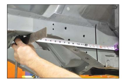
15. Continue marking the cut lines along the inner fender. From the radiator core support to the shock tower overlap seam forward of the tower. And from the 15" line forward to the tower overlap seam.
