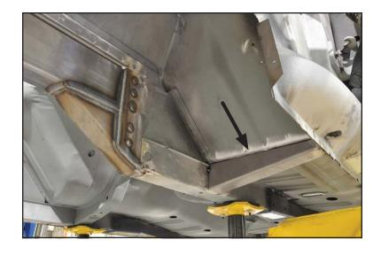
56. Frame Gusset (with torque box) - Test fit, prep for weld, then stitch weld along edges.
