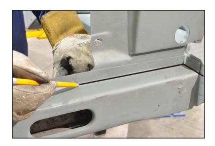
17. Mark the lower control arm mount along the inside corner to just above the curved area.
