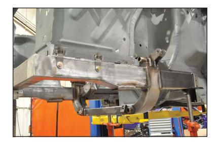
33. Close up any gaps along the outside of the rail before securely tack welding the top and bottom corners of the main frame rail.
