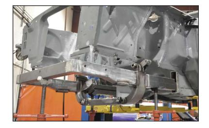
31. Once the rear of the subframe is raised completely into position, install the bolts through the alignment tabs.
