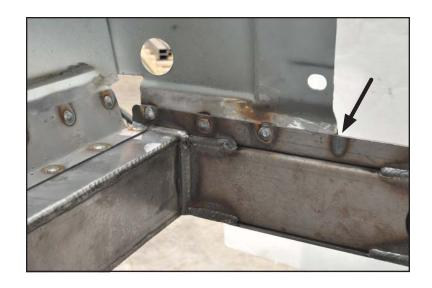
53. A coarse scotch brite pad can be used to bring the welds flush.
