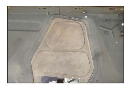
Some installations may require the opening be trimmed to clear the top bead-rolled edge. For these, Cut a horizontal line tangent to the highest radius to meet the other side of the opening.
