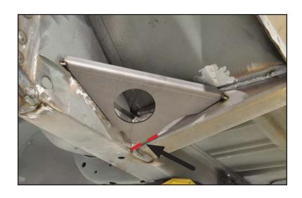
58. Once fit, prep for weld, then stitch weld along edges.
