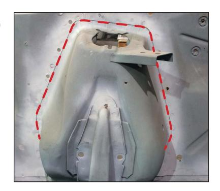
38. From the outside we're left with a doublethick flange on which to weld the tower delete panels.
