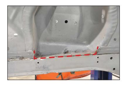
22. Cut up and around the shock tower along the line shown. The bottom legs of this cut must meet the cuts along the inner fender and frame rail.
