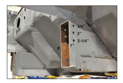
**29. Weld Preparation** - Use a scotch brite wheel to clean the following areas down to bare metal.
