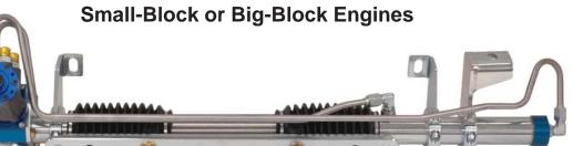
**Description:** High-clearance power TCP Rack & Pinion with mounting brackets and hardware ONLY. Bracket and center-link combination increases oil-pan and exhaust header clearance. **This product requires installation of bump steer kit (TCP TIER-XX) to maintain correct steering geometry.**
