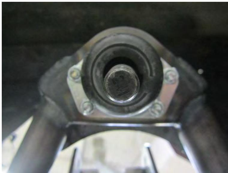
**Upper Ball Joint Installed, Figure 20A**
