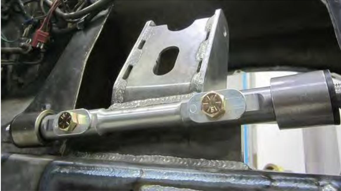
**Fully Assemble Upper Control Arm with 0" Control Arm Slugs, Figure 21D**
