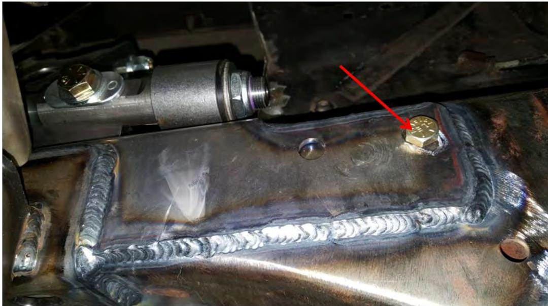
Use OEM 3/8" Dia. Idler Arm Bolt, in Rear Hole of Shock Tower Mount to locate. Mounts in Factory Frame Hole.
