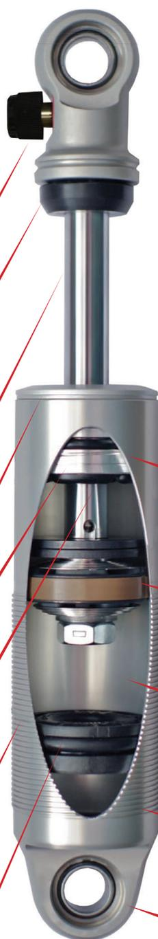
Mono-tube design allows large piston for superior oil control – increases ride quality and handling performance
