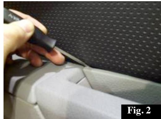
4. Using a panel removal tool pry the switch plate away from the door panel and disconnect wiring. Fig. 3
