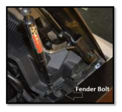
2.) Install Body Bracket w/ball mount pointing toward the engine and located nearest to the windshield.
