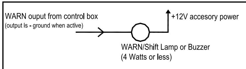
If you need the warn output to be “active high” or provide a +12V voltage to power something larger than 4 Watt, a standard 12V relay such as Dakota Digital RLY-1 can be used to accomplish this.
