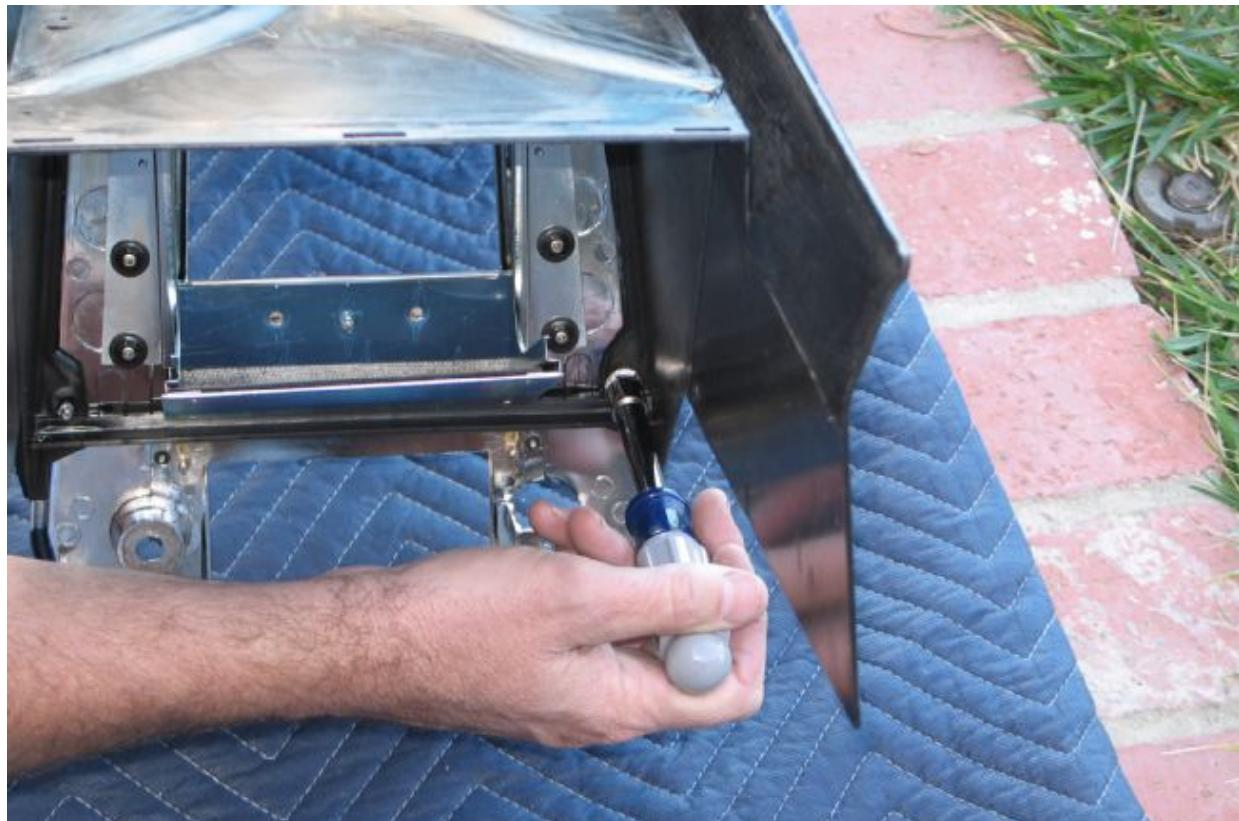
**02.** Next, remove the four speed nuts on the backside of the radio plate . . .
