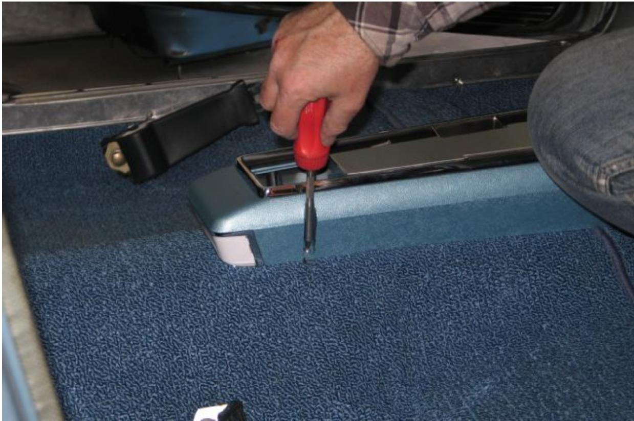
**32.** With the light wiring harnesses and shifter-to-PRNDL rod connected underneath the console, complete the installation by using the same screws that held the old console in place. Step back and take a look at the outstanding results you'll see, like we show at the beginning of this how-to. Once the console is in place, reinstall the shifter handle, finish trimming the carpet, and install the sill plates and seats.
