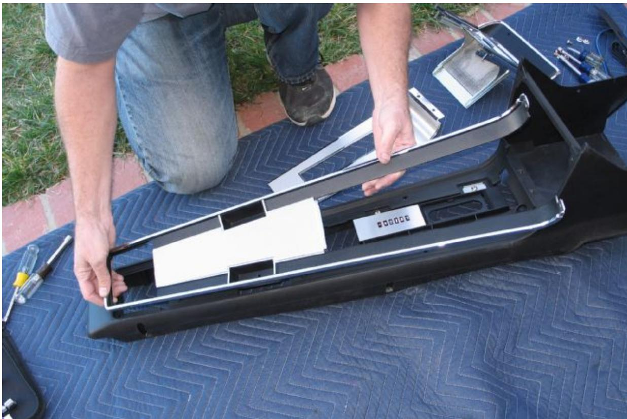
**05.** With the six speed nuts removed from the underside of the console a few steps ago, this main trim overlay that also houses the seatbelt-buckle storage bins is removed as shown.
