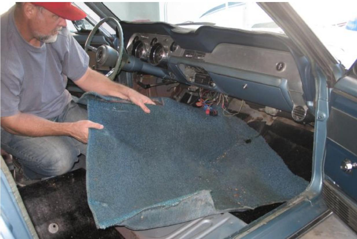
**19.** With the old console and seats removed the old carpet is removed. Now that the crummy old carpet is out, it is a good time to vacuum out the floor pans.
