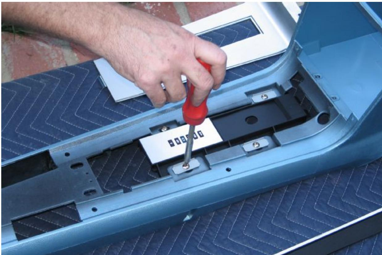
09. Freshly painted in light blue and after the final coat is allowed to dry, the console is then reassembled by reinstalling the shift PRNDL and its four screws.
