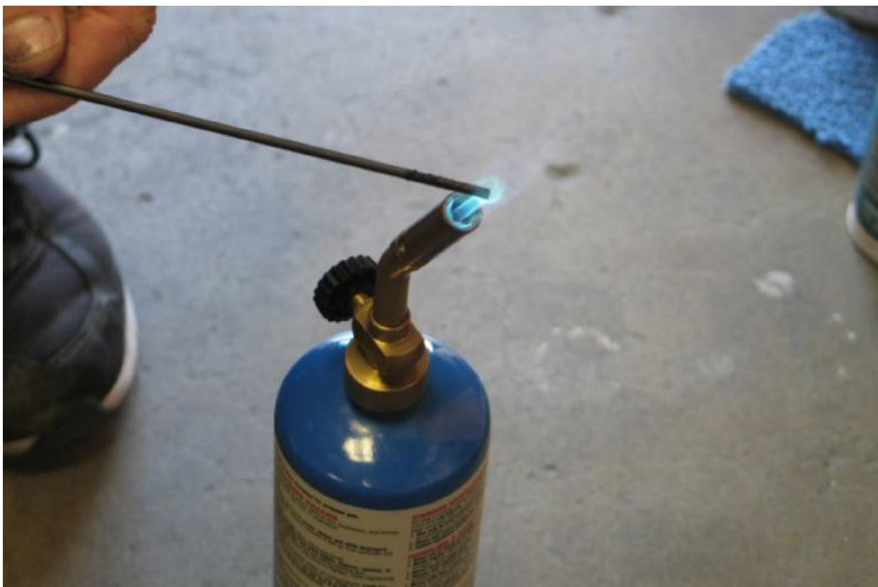
**30.** Our “heat the punch with a map torch” trick worked as good for locating the console-mounting holes as it did for the seatbelts. Get it hot . . .
