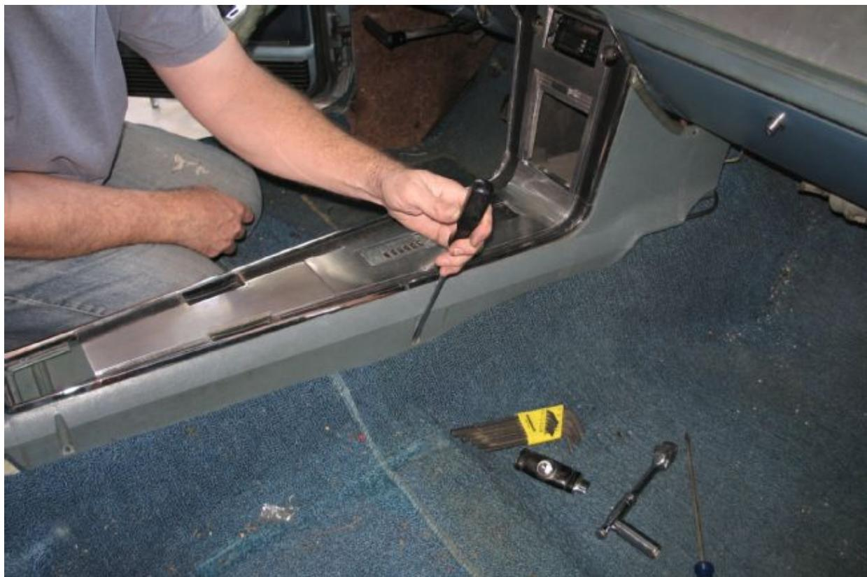
15. With the shift handle removed, the screws that hold the console in place are removed as shown. Of the four screws that hold the console to the floor, strangely only three were present in this car from the factory.
