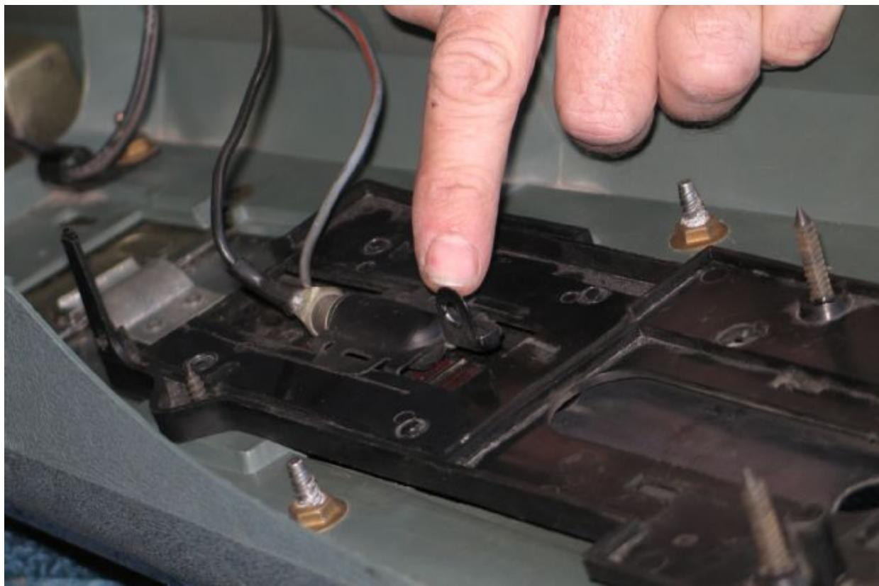
17. This opening is where the plastic rod connects to the PRNDL in order for it to move with the shifter, since the PRNDL is mounted behind the shifter rather than alongside it.
