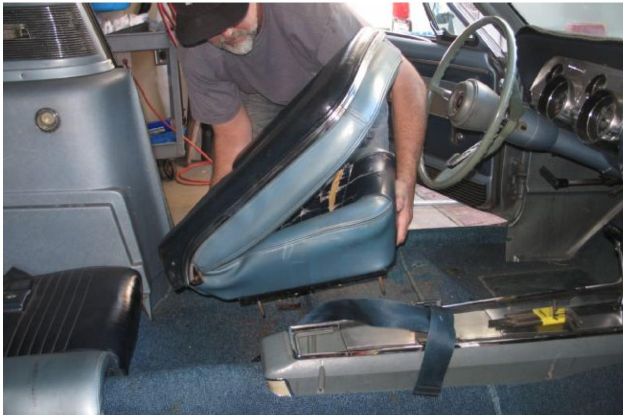
13. With the console all back together and ready to install, we set it aside and started removing the car's seats and carpet. As you can see, the seat covers in this car are pretty ratty and will soon be recovered. Remove the four nuts from under the car that hold the seats in place and they lift out.
