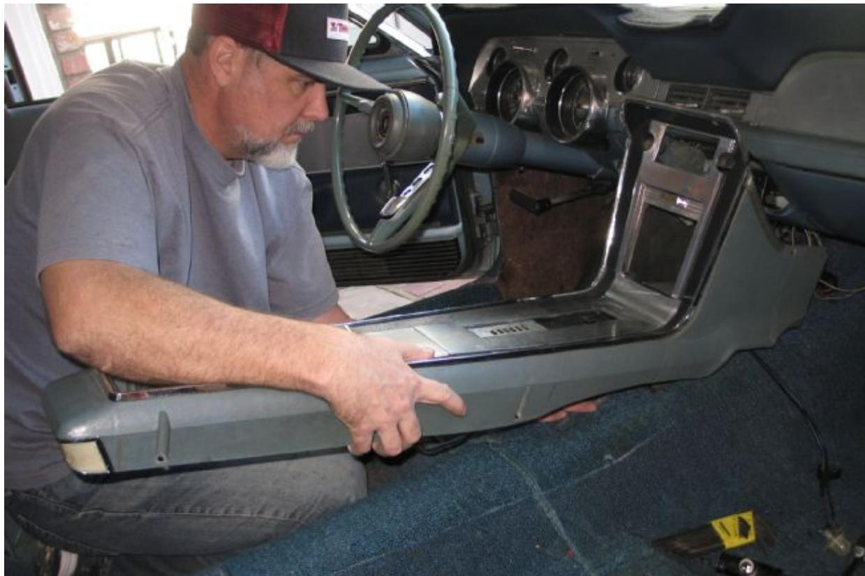
16. This car's original radio was long gone, so once the mounting screws were removed the old console was ready to come out. If a car has the radio still in place it will need to be separated from the mounting plate, which is at the front
