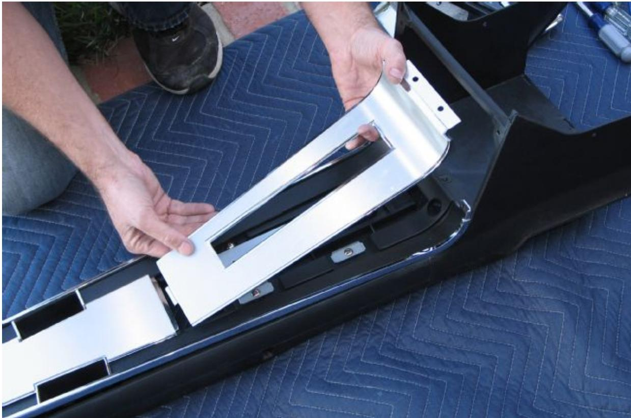
04. Two Philips head screws have been unscrewed to allow this part of the console trim overlay to be removed. The screw holes are visible at the front of this piece. Once they are removed and the radio plate is out, this piece that surrounds the shifter can be removed as shown.
