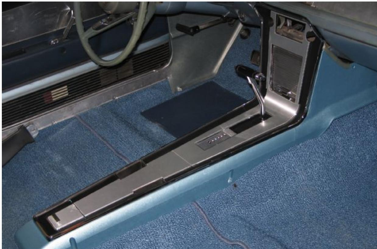
Here is the completed console installation in our 1967 fastback. Combined with new carpeting, it really looks good. The ACP console is a very accurate reproduction that comes about 98 percent assembled. We disassembled it to paint the main plastic body of the console, which doesn't have to be done if your car has a black interior.
