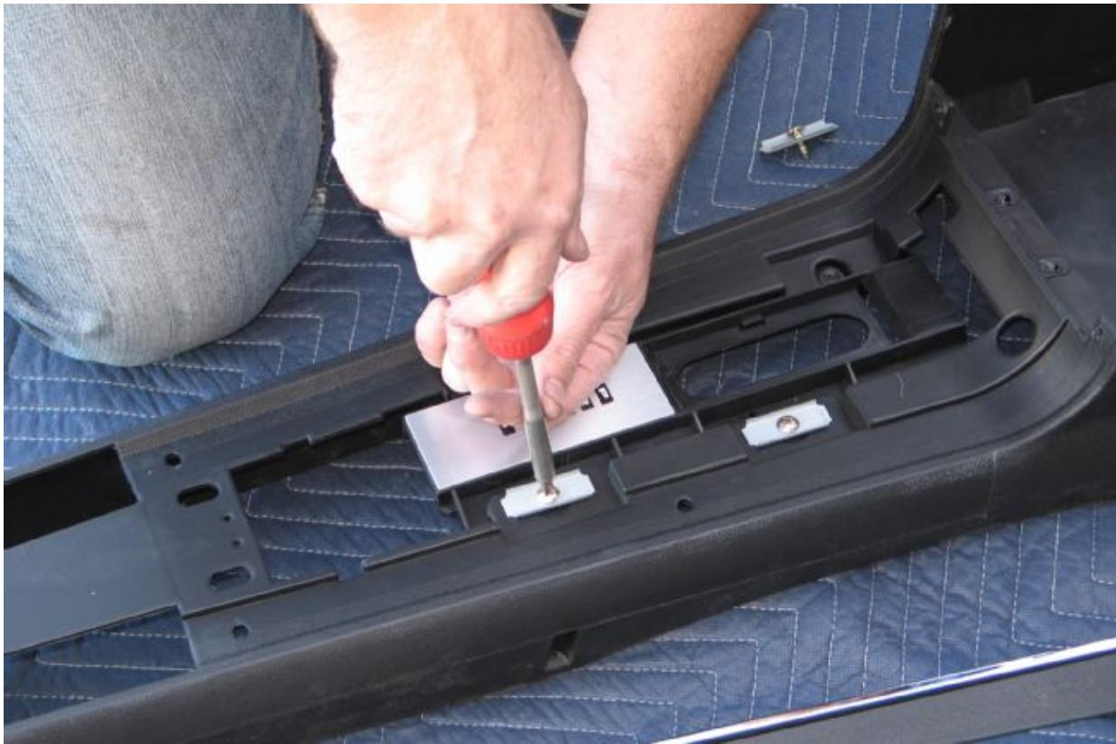
**06.** Remove the four Philips head screws that hold the shift-indicator PRNDL in place, and it comes off of the plastic console body. Once this and the light at the back of the console are removed, the body is down to the bare plastic and is painted in one step.
