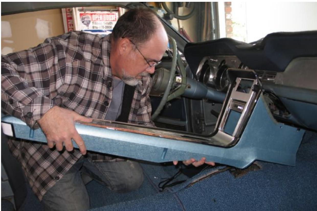
29. Now the console fits properly after the shifter was carefully threaded through the shifter cover in the console. Although it set into place as shown, keep in mind the light connections and shifter-to-PRNDL rod that needs to be connected before it's screwed into place on the driveshaft tunnel. These tasks need to be completed with the console held up while you work underneath it.
