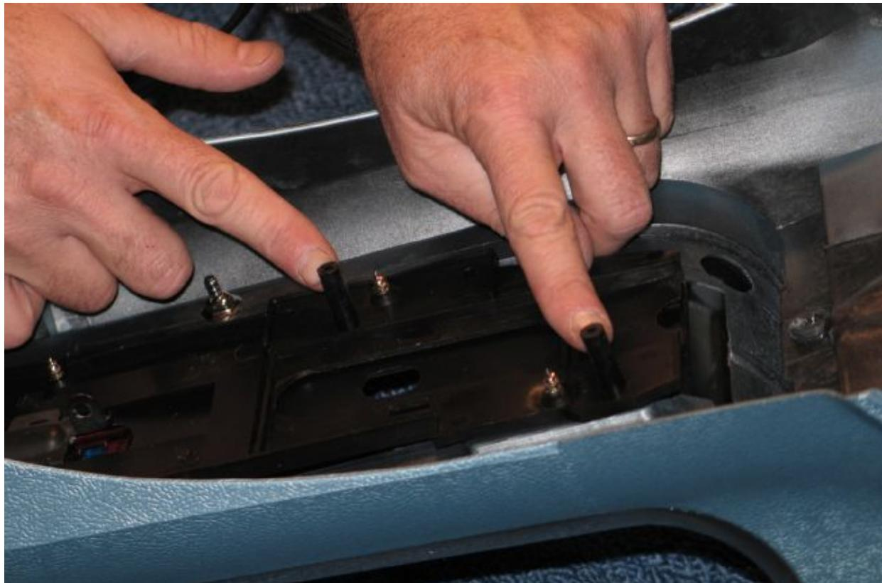
24. These orientation pins are on the new (and old) console to allow it to fit correctly on the shifter. They fit into the openings in place on . . .
