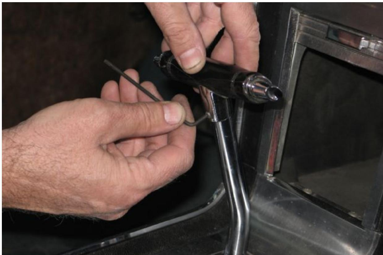
14. Removing the old console commenced with loosening the set-screw on the shifter handle so it could be removed.
