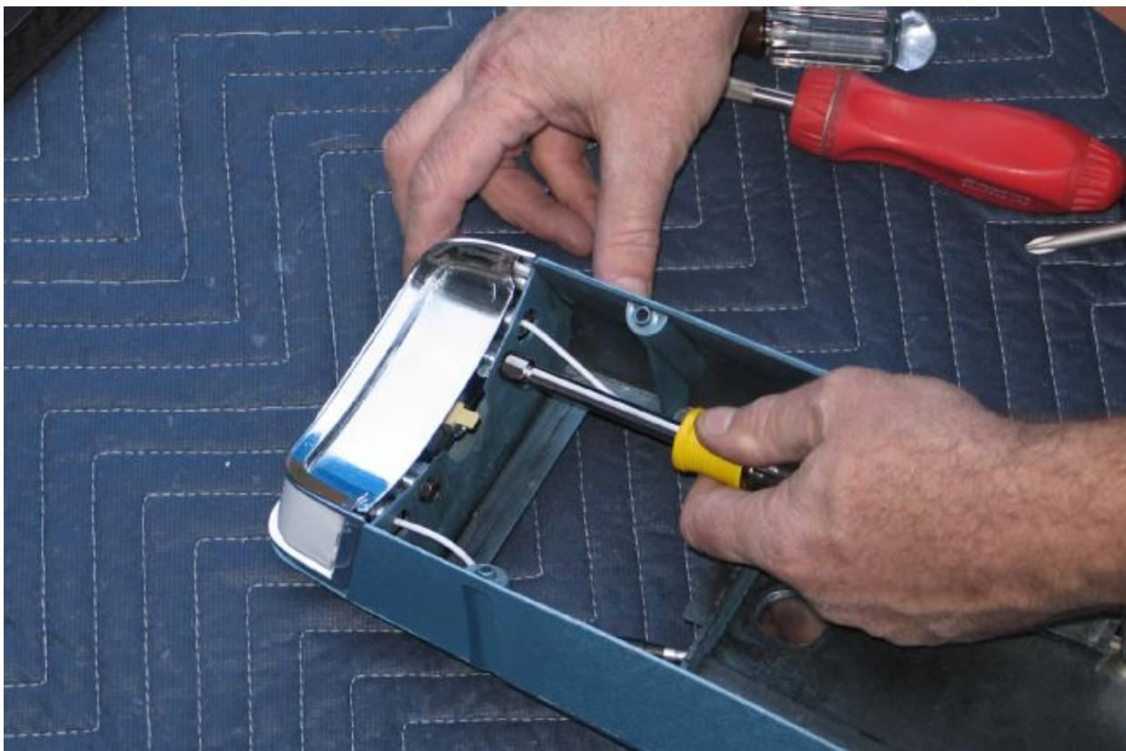
10. Not shown being removed, this is the light mounted at the back of the console being reinstalled.
