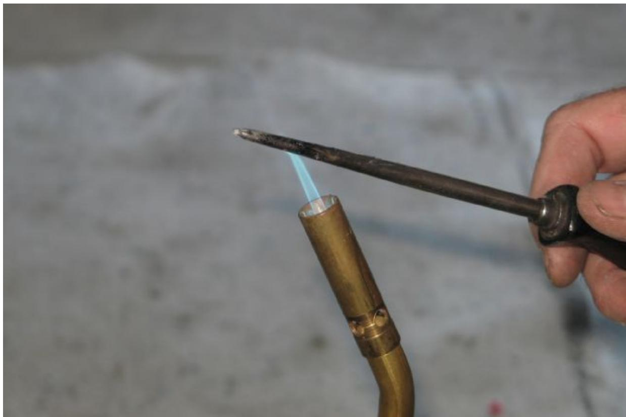
22. With the carpet roughly in place, we came up with a little trick for making the seatbelt holes, which are usually a hassle to cut. It might be a little funky, but it worked great for us. First we poked a punch through the carpet from underneath the car. Then, as shown here, we heated up the punch real good with a map torch.
