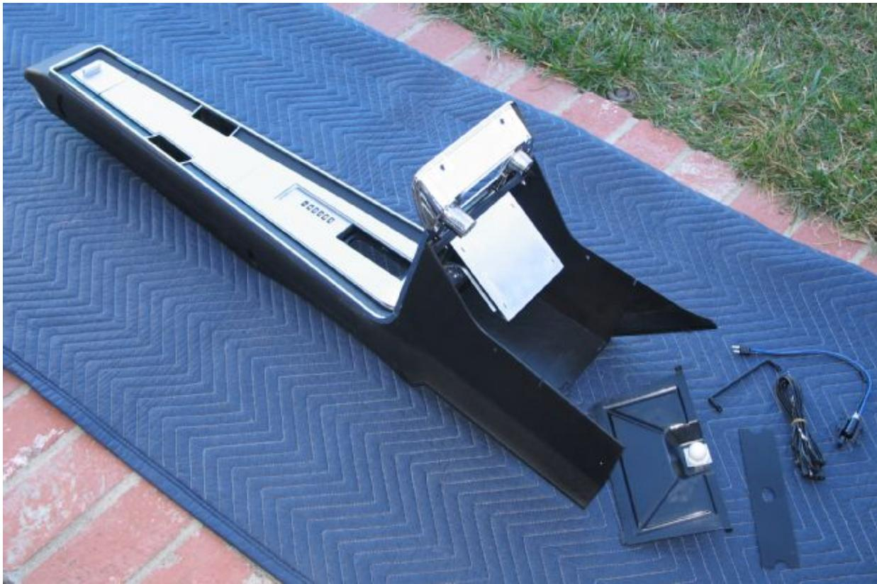
As shown here, the included parts not installed are the back wall (with light) for the console's front storage compartment, the shifter cover for the shift handle that goes in front of the "prindle" (PRNDL) shifter-position indicator, two wiring harnesses for the various lights that are in the console, and the plastic rod that connects the
