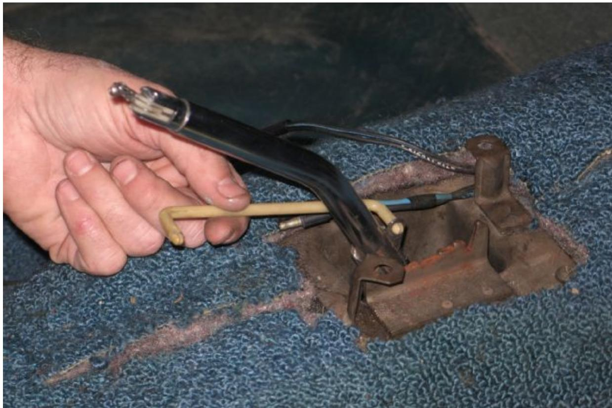
18. Here is the bar with the console removed and it still attached to the shifter. When you're installing the new console, it needs to be connected with the console in place but before it's lowered into final position. The console
