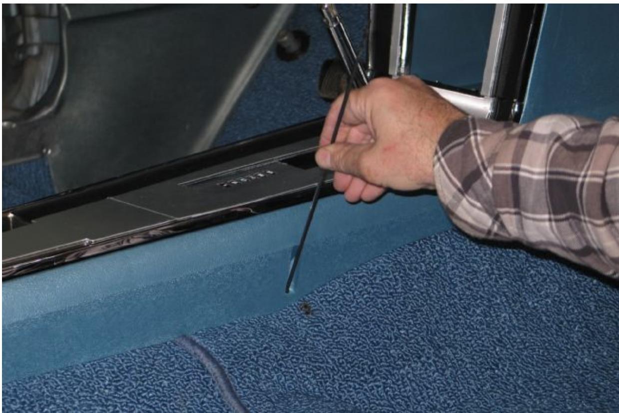
**31. . .** and use the punch to melt away the carpet to allow the much smaller (than seatbelt bolts) Philips screws that attach the console to the tunnel to grab hold of the car's floorpan. Note also that we used the console itself as a template to help get the punch to fit through the holes in the floor.
