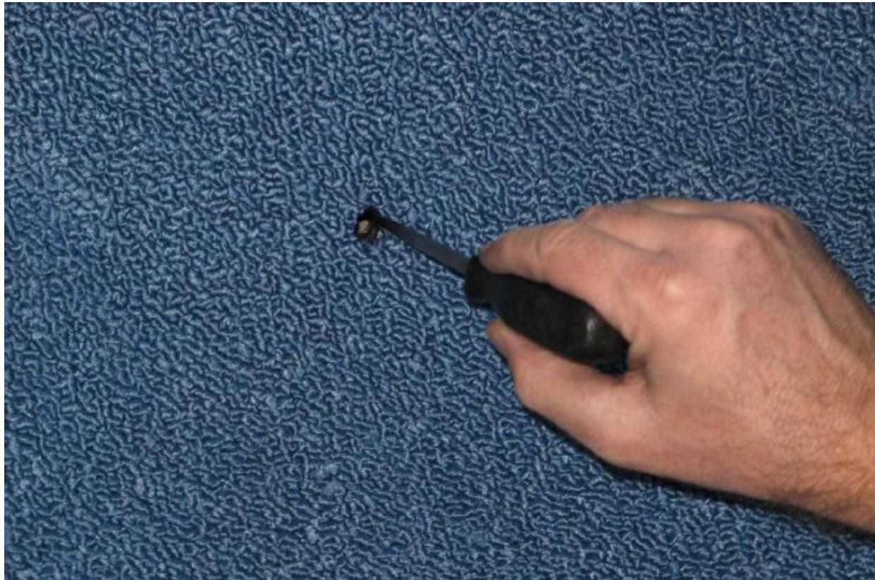
23. Then with the punch good and hot, we used it to carefully melt the carpet exactly where we wanted it so it wouldn't be so difficult to get the seatbelt bolts started. The hot punch perfectly melted away the carpet to create just the right opening, as shown, to make reinstalling the seat belts a snap, which is the next thing we did.
