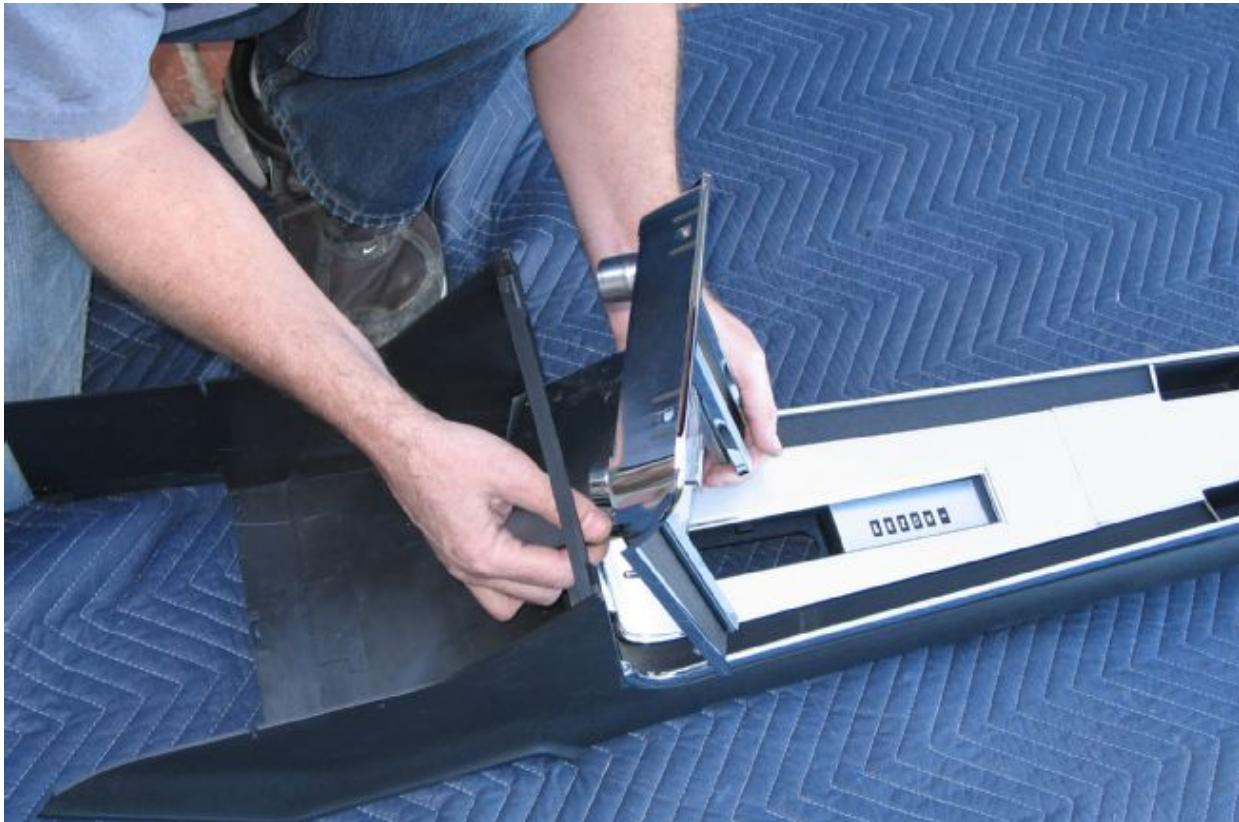
03. . . and the plate can then be removed from the console body.
