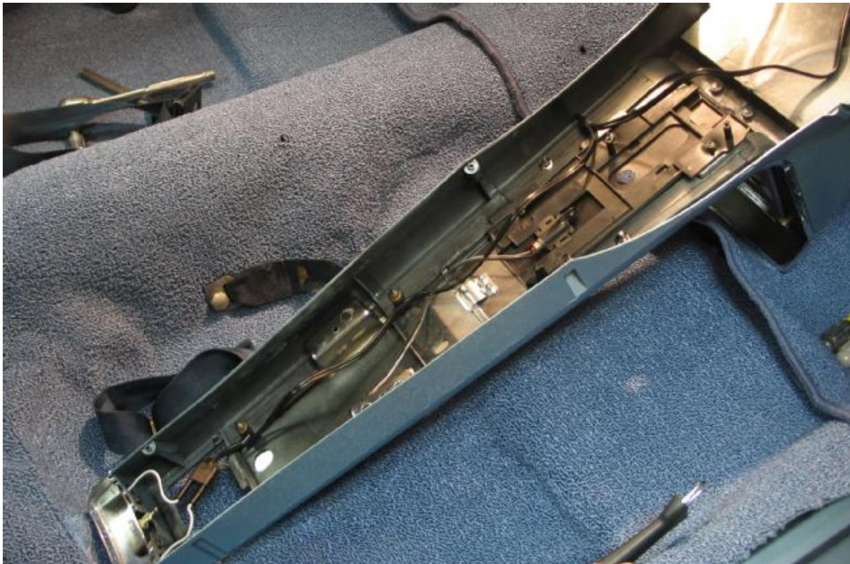
12. With the wiring that comes with the new console and that in our original console, we were able to wire up the three lights in the console as shown. They include the rear courtesy light, one for the PRNDL, and another for the front storage compartment.
