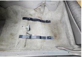
8. Using the factory hardware from step 2, secure the front of the new Stifflers seat rail extenders. Torque to 25-34 ft-lbs.
