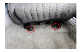
3. Locate the tilt lever on the back of the seat to tilt the seat forward. Now, relocate the sliding seat track lever in front of the seat, and slide the seat all the way to the forward position.
