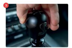
INSTALL THE SHIFT KNOB ONTO THE THREADED INSERT. IF THE ENGRAVING IS CROOKED, REMOVE THE SHIFT KNOB & ADJUST THE JAM NUT & THREADED INSERT
