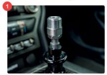
INSTALL JAM NUT, THEN THREADED INSERT ONTO THE SHIFTER.
