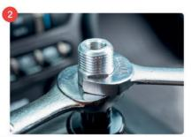
TIGHTEN THE JAM NUT & THREADED INSERT TOGETHER USING 1-2 WRENCH(ES). IF NOT TIGHTENED PROPERLY INSERT MAY GET STUCK IN THE SHIFT KNOB
