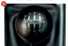
REINSTALL THE SHIFT KNOB ONTO THE THREADED INSERT. REPEAT UNTIL ENGRAVING IS ALIGNED STRAIGHT.
