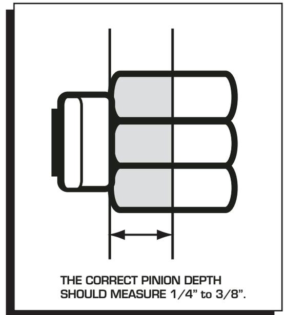
THE CORRECT PINION DEPTH SHOULD MEASURE 1/4" to 3/8".
