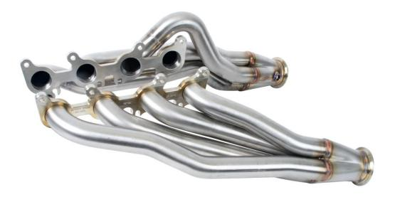
**NOTE**: When installing these headers in the DSE Aluma-Frame, it is required that you use the Detroit Speed Ford Modular Engine Mount Kit P/N: 060420DS.
