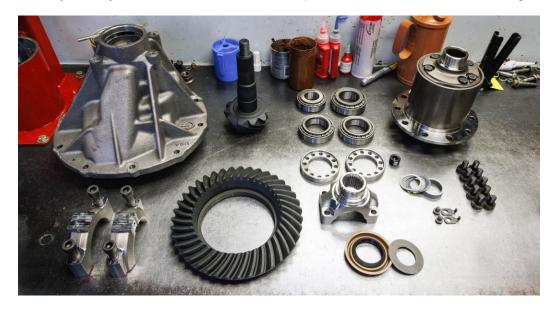
The Ford 8.8 has a long history of reliably handling punishment in drag competition and other demanding environments, especially when prepared with premium components. The FN988 comes with a 31-spline Eaton Truetrac differential, giving it strength roughly equivalent to that of any other rear end with 31-spline axles, says
