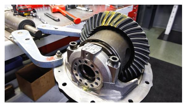
One of the main differences between the 8.8 and the 9-inch is the pinion location. The 9-inch's pinion is offset lower on the ring gear than that of the 8.8. This low position adds strength, but it saps power and creates noise, making the 8.8 relatively silent by comparison. Further adding to the 8.8's quietness is the availability of OEM gearsets for it.
