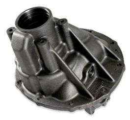
The FN988's dropout case is based on the general configuration of the 9-inch, and it fits 9-inch axle housings. But it's an all-new design created by GearFX and Detroit Speed. This made-in-USA nodular-iron case accepts all standard 8.8-inch components. Visible here are pre-drilled holes on the front pinion area for mounting accessories such as speed sensors or pumps.
