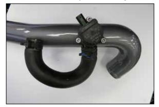
9. Install the BOV onto the K&N hot side charge tube and secure with the factory hardware removed in the previous step. Install the factory BOV hose onto the K&N hot side charge tube.
