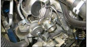
11. Install the provided step coupler into the turbo outlet with the provided clamps, do not tighten the clamps.
