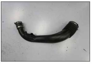
4. Loosen the hose clamp the secures the factory intake tube to the turbo inlet and then remove the intake tube from the vehicle.
