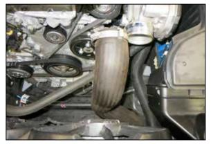
5. Loosen the hose clamps that secure cold side charge hose to the throttle body and inter cooler and then remove the cold side charge hose from the vehicle.
