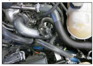
13. Install the K&N hot side charge tube into the couplers, align the tube for best fit and then tighten all the hose clamps. Reconnect the BOV electrical connection.
