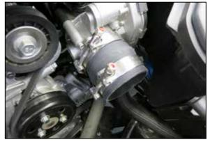
14. Install the provided hump coupler onto the throttle body with the provided clamps, do not tighten the clamps.
