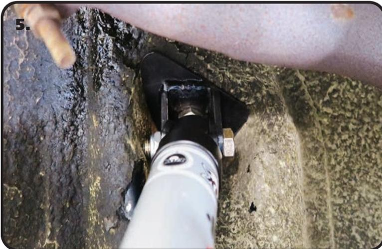
**5.** The Shock is mounted in the Upper Mount with the BODY UP. It is held in place with a 1/2"-20 x 2 1/4" Hex Bolt & 1/2"-20 Nylok. If the threads of the bolt would happen to touch the floor pan of the car, a 1/2" Flat Washer can be installed under the head of the bolt.
