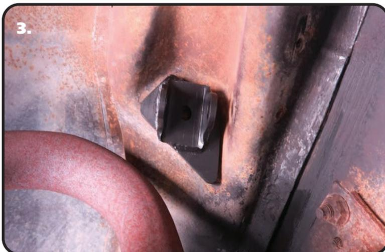
3. Install the Passenger Shock Mount will be installed in the OEM location. The Shock Mount is shaped to fit the body and will only fit into the OEM location one way. Install the mount into the OEM location with the Stud sticking through the OEM shock hole. Have someone hold the mount in place while installing the top support and mounting hardware,
