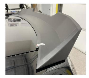
2. Install spoiler onto the trunk lid making sure all 4 threaded rods are protruding through the trunk lid.
