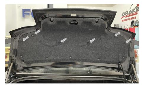
1. Open trunk and remove 6 plastic clips using clip removal tool.
