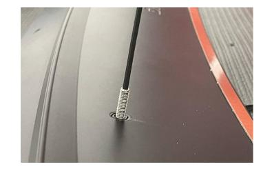
1. Apply Loctite and thread (x4) M6 threaded studs into spoiler using a 3mm Allen wrench, leaving the majority unthreaded as shown above.
