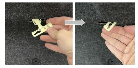
2. Push trunk release latch through slit in trunk liner.
