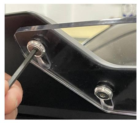
1. Install Lexan flap with (x6) billet washers and (x6) flat head screws as shown using a 4mm Allen wrench. Be sure not to overtighten.
