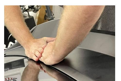
5. Push downward at multiple points on the front edge of the spoiler, pressing the tape into the trunk lid. Hold for a few seconds at each location for the tape to fully adhere.
