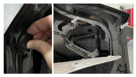
3. Peel trunk liner forward and remove (x2) plastic caps towards the outside of trunk lid using clip removal tool (outside gray arrow shown above).
