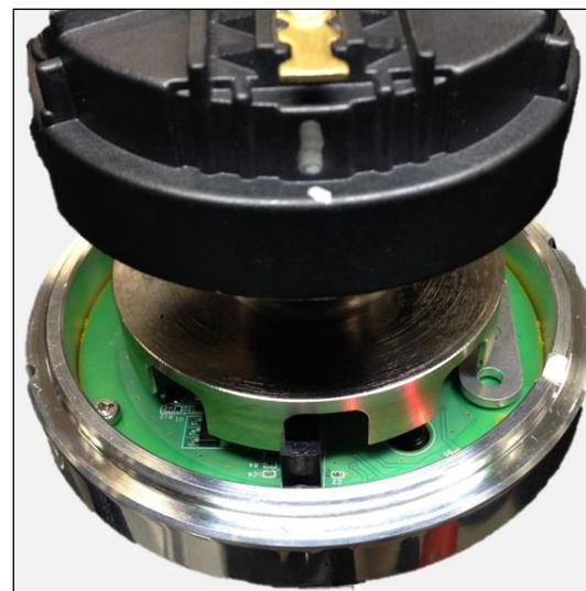
Then slowly turn the housing **counter-clockwise** until the Crank LED comes back **ON** (**Figure 4**). Stop at this point. This will position the distributor close to where it needs to be. Install and snug the distributor clamp down at this point.
