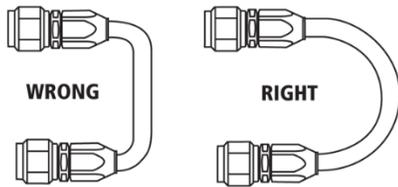
Keep the bend radius of the hose as large as possible to avoid collapsing of the hose and restriction of flow. Follow catalog specs on minimum bend radii.
