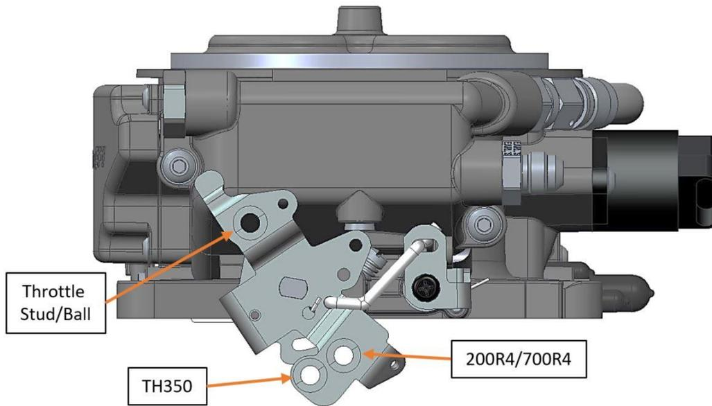
4. Reconnect the throttle and if applicable transmission kick-down linkage. Be sure to check for any binding conditions and correct before proceeding. Poorly routed throttle cables & linkages can cause throttle pedal issues.
