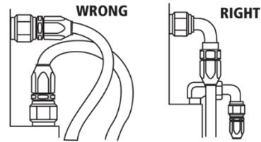
Use elbows and adapters in the installation to relieve strain on the assembly and to provide easier and neater installation that are accessible for inspection and maintenance.
