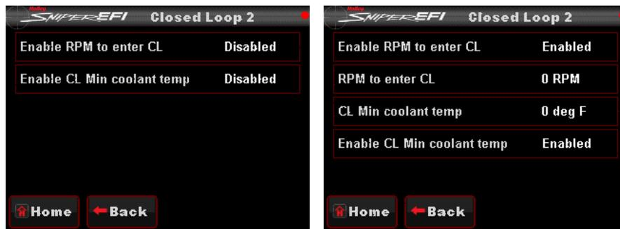
**Enable RPM to enter CL:** This setting is disabled by default. If an extremely large camshaft is used (specs only typically found on race camshafts), the overlap sometimes causes a "false lean" reading at low RPM. In these cases, it may be required to enable this function and put in a value of above idle RPM so the system operates open loop below this RPM setting.
