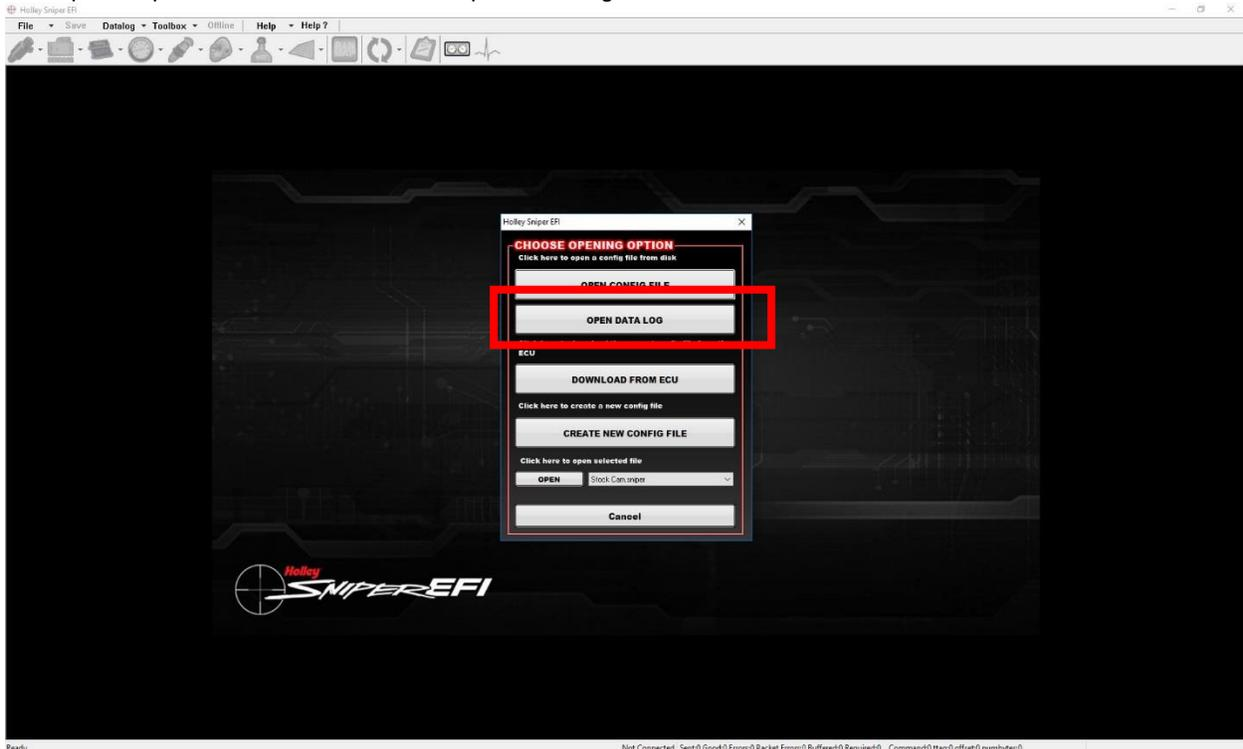
Navigate to the data log on the SD card the file will be in the “Saved Datalogs” folder on the SD card. Next, click the “Open” Button. The data log will open to be viewed.
