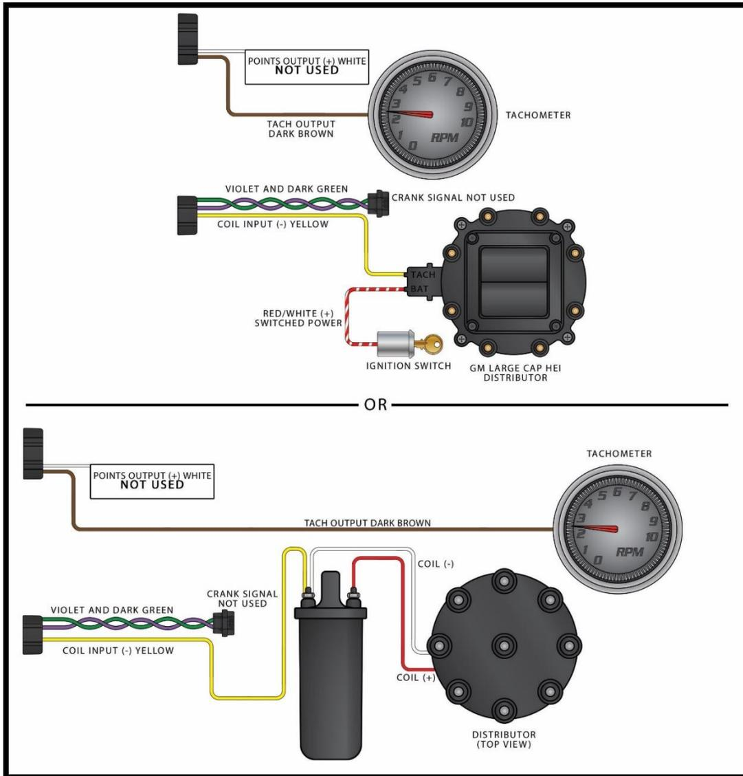
**WARNING!** Do NOT use this input if you are using an aftermarket Capacitive Discharge (CD) ignition system such as a MSD, Mallory, or others. The ECU will be damaged if you connect to a capacitive discharge type ignition coil.
