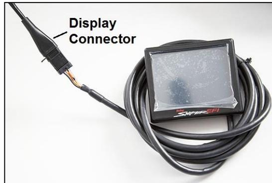
**Note: If the 3.5" Touch Screen LCD Display needs to be unhooked from the Sniper EFI. Depress the lock tab on the male side of the connector as show in the following pictures.**
