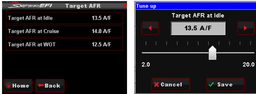
**Idle Air/Fuel Ratio** – Typically between 13.5 and 15.0. Engines with larger cams may need a richer setting for smoothest idle.
