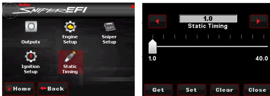
**Get Icon:** If static timing has been set and user has navigated to another screen in the handheld, press the "Get" icon to view what the static timing has been set to.
