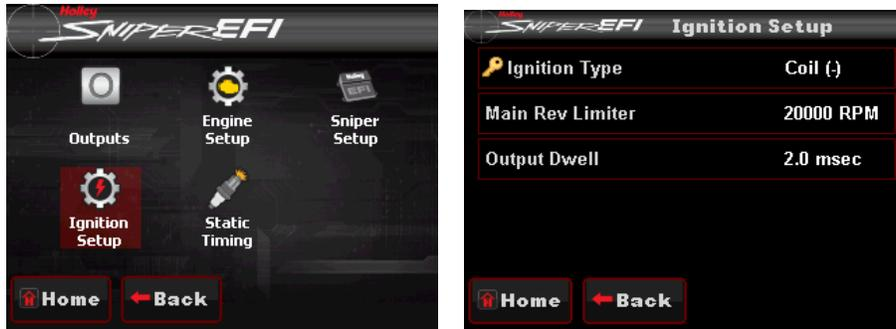
**Ignition Type:** Change the calibration for different ignition setups
