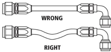
In straight hose installations, allow enough slack in the hose line to provide for changes in length that will occur when pressure is applied. This change in length can be from +2% to -4%.
