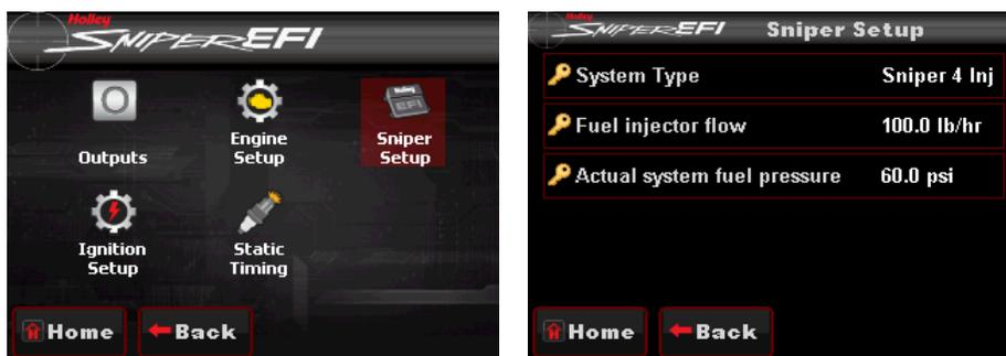
**System Type:** Change the calibration for different part numbers within the Sniper EFI Family
