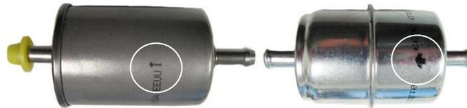
**WARNING!** Ensure both filters are installed in the proper direction. A flow direction arrow is printed on the side of the filter to indicate the direction of fuel flow. Failure to do so will result in a system malfunction.
