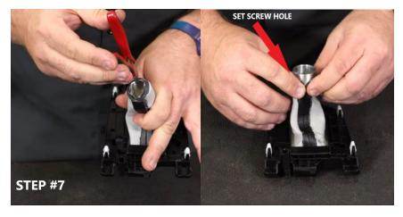
set screw hole in the side of the shift handle.
