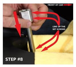
Step 8: Time to install the Shelby Shifter handle retainer. Note: make sure to lay a rag or something down in the shifter location in the center console to prevent droping the small screws.
