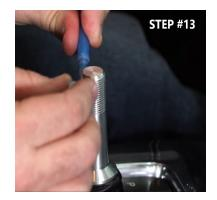
Step 13: If you have the Shelby "T" handle shifter, place a generous amount of lock tight on the threads of the shift handle. Then thread the "T" Handle onto the shifter handle until it is as far as it will go while keeping the logo straight.
