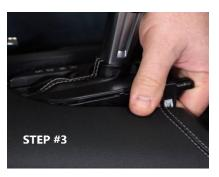
Step 3: Remove the base plate, that is held down by clips, by pulling up on the front and use a plastic pry bar to assist with the sides. Step 3a: Unplug the base plate. The plug is located on the front of the base plate. You will have to press the tab, then pull it down and out of the base plate
