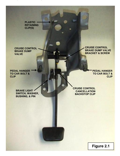
2. Remove the bolt holding the brake pedal in the assembly.
