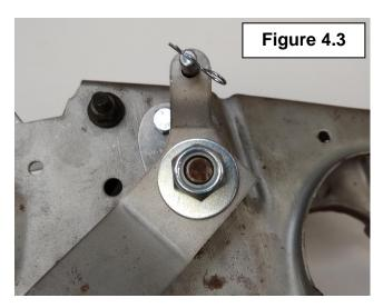
11. Install the clutch switch bracket to the pedal frame using the #10-24 x 3/8" button head screw and locknut.
