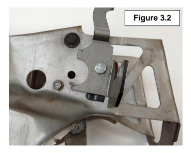
7. Reinstall the brake pedal using the original hardware, but this time routing through the hole in the clutch stop bracket.
