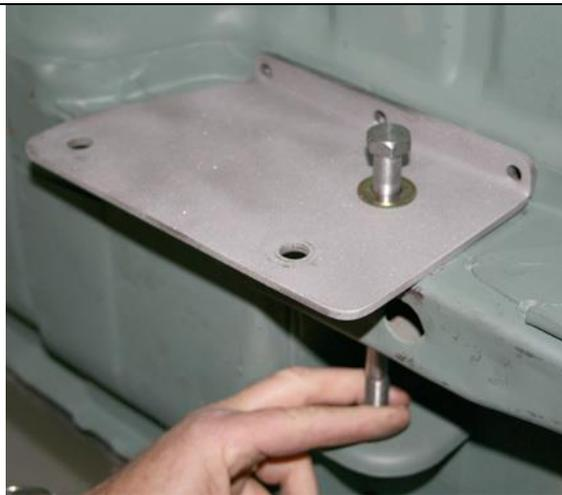
With all the old suspension removed, start by installing the rear inner sub-frame support plates (L&R) aligned with the front stock leaf spring hole using the ½ inch by 6½ inch bolts, washers and nuts that are furnished and lightly tighten.
