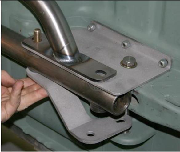
Push the two rear connector  $\frac{1}{2}$  by  $3\frac{1}{2}$  inch bolts through the front holes of the stiffener flanges, install nuts and washers and leave loose.
