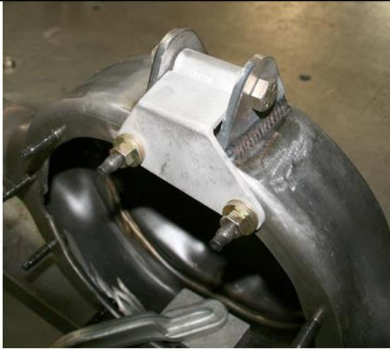
The torque arm tabs are welded on by using the supplied fixture tool. Bolt fixture to the lowest 2 third member bolts flat against the housing flange. Bolt on the two supplied tabs using the 1/2 by 3 1/2 inch bolt and with the longer tab to the passenger side of the housing. Bottom of tabs may need sanding to fit. Weld outside and wrap welds also to the inside.
