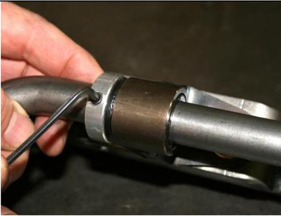
Center the bar on the cross member and slide the aluminum rings on the sway bar with set screws installed up against the urethane bushing flange, and tighten set screws.
