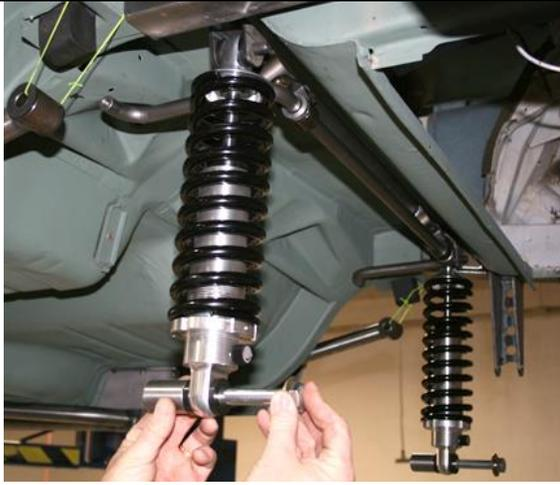
Install the 5/8 by 6 inch bolt with washer on the shock and 1 3/4 inch spacer on the bolt.
