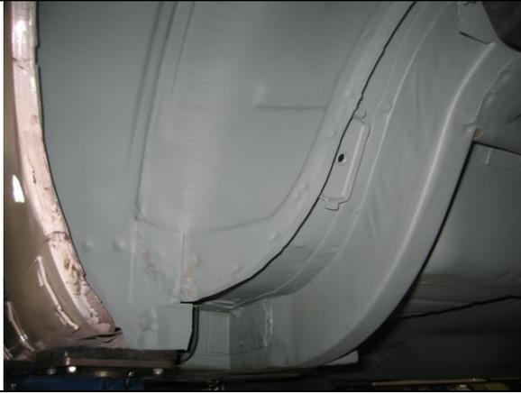
**Note:** The Mustang wheel well curves outward about 2 inches in the front. This limits the size of the rear tire you can install.
