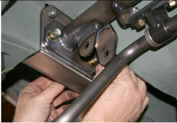
Bolt in with the four 3/8 by 3 inch bolts, washers, nuts and tighten. Note: The flanges on the ends of the cross member are slotted and angled the same as the frame to allow the cross member to be adjusted fore or aft slightly to allow cross member to be parallel to the rear axle assembly.
