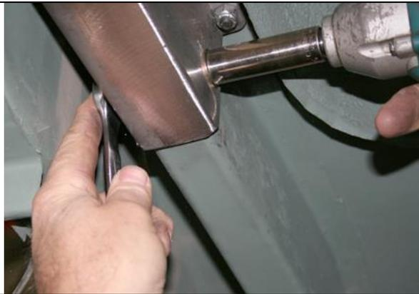
Next, install the rear 3/8 by 2 1/2 inch bolt through the channel bracket and tighten.
