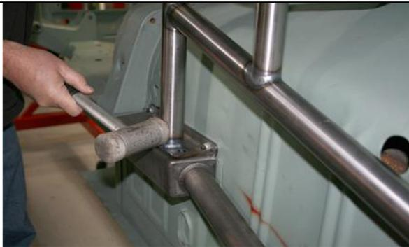
Lift the torque arm cross member/frame stiffener up between the rails; lightly tap cross member into place between the sub-frame channels.
