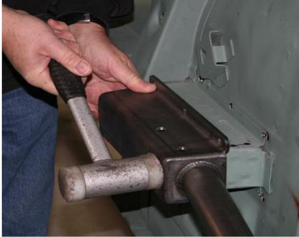
Tap the sub-frame connector front channel over the stock frame rail until flush with the floor. Note: You may have to do a little hammer work on the stock frame rails to square them up to install channels. My 67 Mustang's rails had taken quite a beating during the last 40 years.
