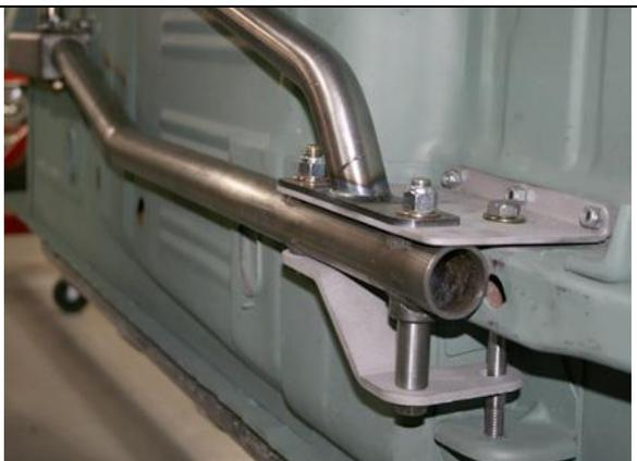
The trailing arm will be installed either in the top hole (stock spring location), street application or the bottom hole, strip application. On this project, we are using the street setup. Install the  $\frac{1}{2}$  by  $5\frac{1}{2}$  inch bolt through the brace, through the  $1\frac{3}{4}$  inch long spacer, through the sub-frame connector, support plate and through the stiffener flange rear hole. Install nut and washer and leave loose.
