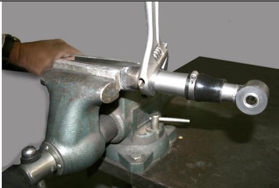
The Torque Arm is shipped with the slider assembly separate to facilitate packaging. The slider has been pre-assembled with Teflon bushings and has been installed in the Torque Arm to check for proper fit. We use anti-seize on the threads to prevent galling. When painting or powder coating the assembly, tape the threads on the slider and plug the hole in the Torque Arm tube.
