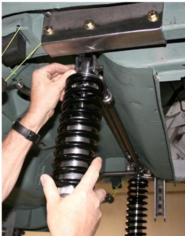
Install the coil-over shocks (250 lb. rate) on the cross member with the 1/2 by 2 3/8 inch button head bolt, washers and half nyloc nuts.
