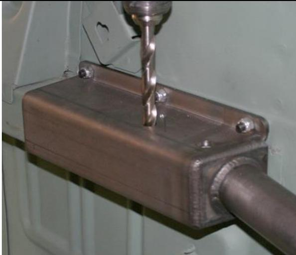
Next, the eight 1/2 inch front side holes in the front sub-frame connector channel have to be drilled in the frame. To keep the holes centers straight, drill from the inside and outside of the rail rather than try to drill all the way through from one side. Hold the drill securely as it will want to grab the thin frame sheet metal.
