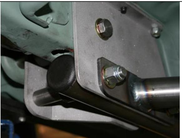
Install the plastic end cap on the end of the sub-frame connector tube by tapping with a hammer after paint or powder coating. Tapering the front ribs on a sander makes installation easier.
