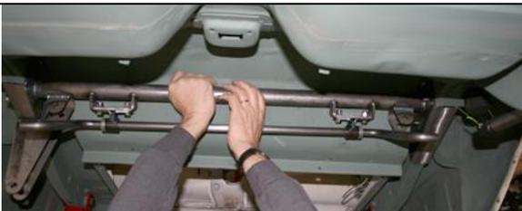
Install the coil-over/sway bar mount cross member between the frame brackets with the coil over mounts and the sway bar brackets towards the rear of the car and the sway bar ends pointing forward.
