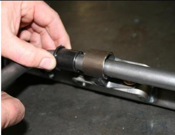
Slide the urethane bushings on and hand press the bushings into the tube brackets.
