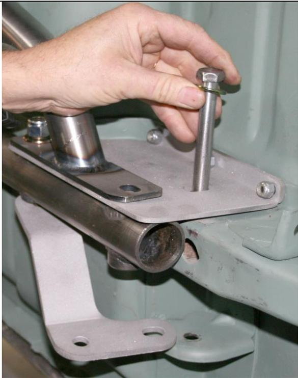
The long  $6\frac{1}{2}$  inch bolt previously installed in the support plate needs to be unbolted and partially pulled out to allow the brace bracket to be rotated into the proper location.
