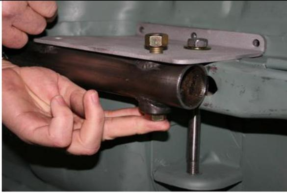
The sub-frame connectors (L&R) are installed by bolting the rear hole of the connector with a 1/2 inch by 3 1/2 inch bolt to the rear hole in the support plates to locate the front channel in the correct location before drilling holes.
