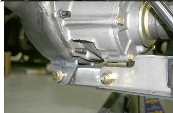
Install the rear of the Torque Arm to the tabs on the bottom of the rear end housing using a 1/2 inch by 3 1/2 inch bolt, washers and nut. Lightly tighten.
