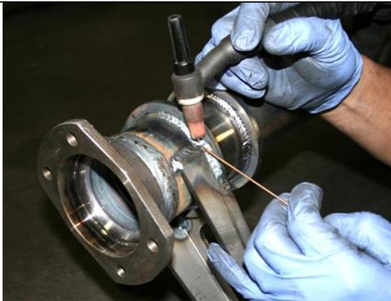
Finish welding axle brackets and panhard bar bracket the full 360 degrees inside and outside.
