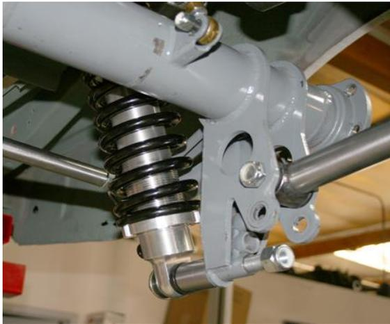
Time to install the axle housing assembly. You can use a hydraulic floor jack under the third member or have a couple of your strong friends, like I did, lift the ends of the housing while I pushed the long 5/8 inch bolts through the lower mounting hole in the axle brackets. I left off the axles and brake kit because of the extra weight. Tighten the 5/8 nyloc nuts.
