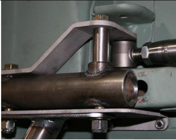
Adjust the trailing arm to 20 1/8 inch centers for a starting point. Install the adjuster end of the trailing arm between the stock inner spring pocket and the brace.
