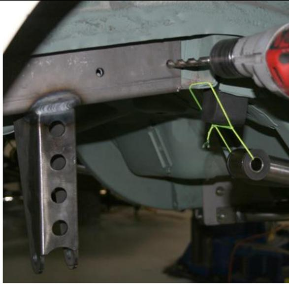
Next the 3/8 inch holes in the sides of the channel brackets need to be drill out. The front holes on both sets of brackets can be drilled from the inside and the outside without using the drill guide plate. Drill the outside holes both sides and the front inside holes from the inside.
