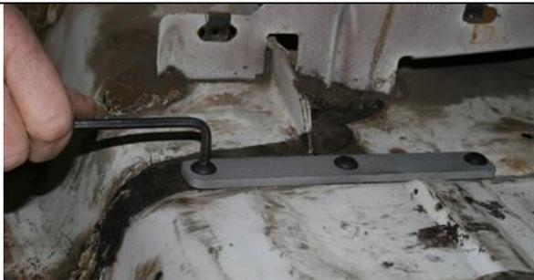
Tighten the 3 button head bolts on the inner frame sub-frame support plates that were left loose. This will pull the connectors up tight against the frame.
