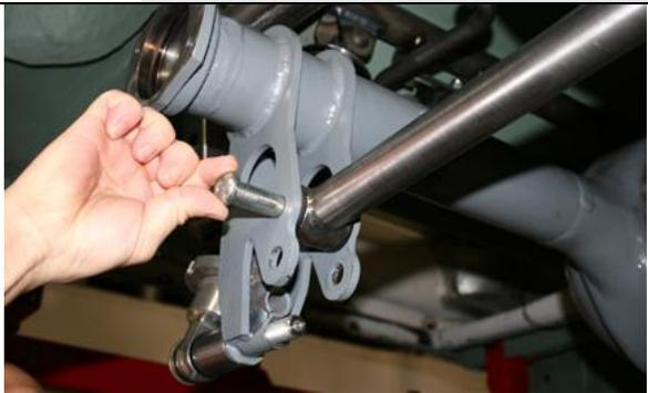
Install the trailing arm bars using the  $\frac{5}{8}$  by  $2\frac{3}{4}$  inch button head bolts and the half nylocs in the top holes in the axle brackets (street), lower hole for strip application.
