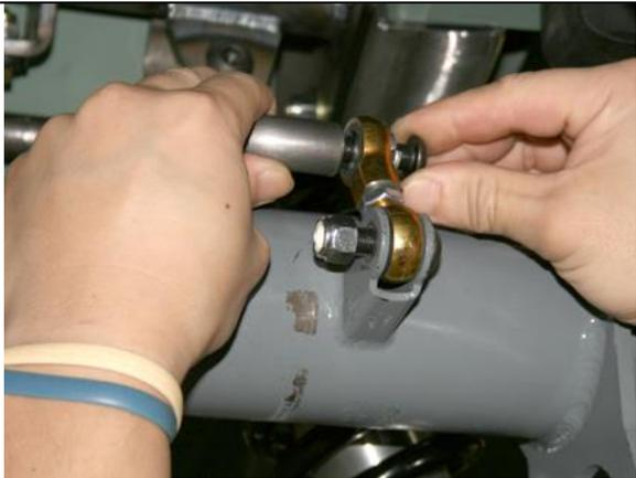
Install the rod end links on the sway bar using the 3/8 by 1/4 inch button head bolt and lock washer. Bolt the bottom of the link to the sway bar bracket on the housing.
