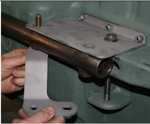
Installation of the torque arm cross member/frame stiffener is next. Remove the two ½ by 3½ inch bolts fastening the rear of the sub-frame connectors to the support plates. Install one of the bolts and washers through the front of the trailing arm brace brackets (L&R) then through the sub-frame connector then partially through the support plate. Let the rear of the plate hang down temporarily. Do both sides.
