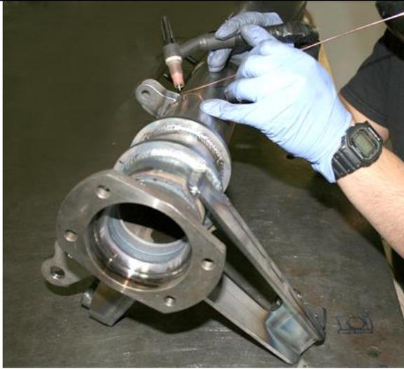
The sway bar brackets are located on the front of the axle tubes at axle centerline on 32.75 centers. Finish welding sway bar brackets and straighten rear housing.
