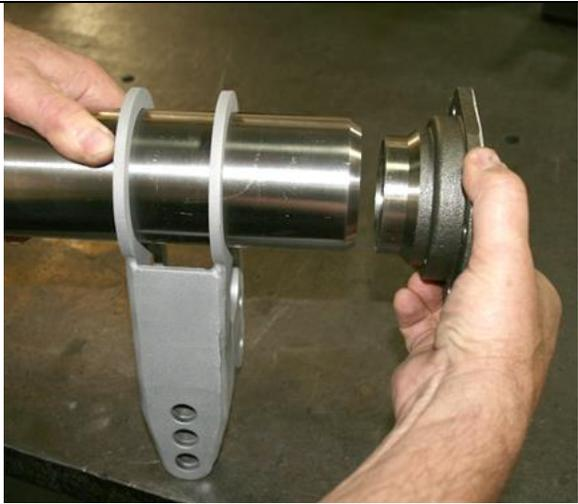
The rear axle brackets, panhard bracket and the sway bar brackets are installed as per the drawing. I would highly recommend getting this done by somebody with experience narrowing rear axle housings. The kit uses a nine inch centered pinion axle housing. Recommended axle bracket installation is to slide the brackets over the axle tubes without the bearing flanges attached rather than cut the brackets and re-weld together on the housing.
