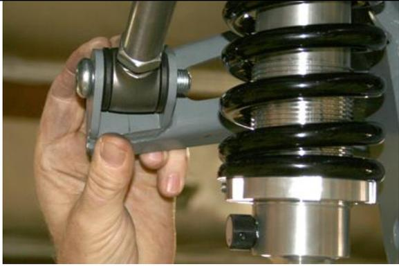
Install the panhard bar next using the 9/16 by 2/4 inch button head bolts and the half nyloc nuts.
