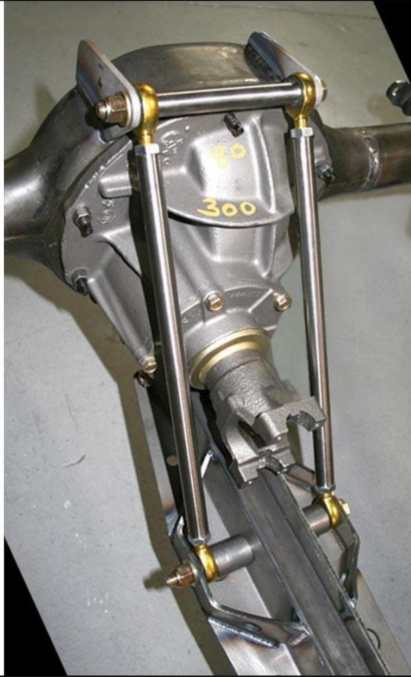
The pinion support tubes have left and right hand rod ends to facilitate pinion angle adjustment. Adjust the tubes to approximately the same length with an equal amount of threads showing on each rod end. Install the tubes with the right hand rod ends on the inside of the top brackets using the 1/2 by 8 inch bolt, washers, 5.2 inch spacer in between rod ends and Nylock nut.
