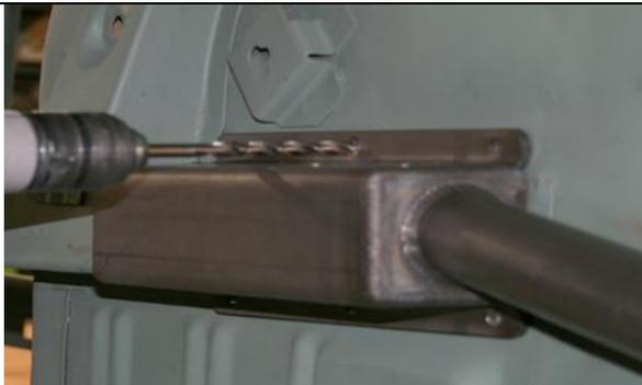
With the sub-frame channel pushed solidly against the floor and the rear of the connector bolted to the support plates, drill the first hole through the floor with a 5/16 drill bit using the channel's holes as a guide pattern.
