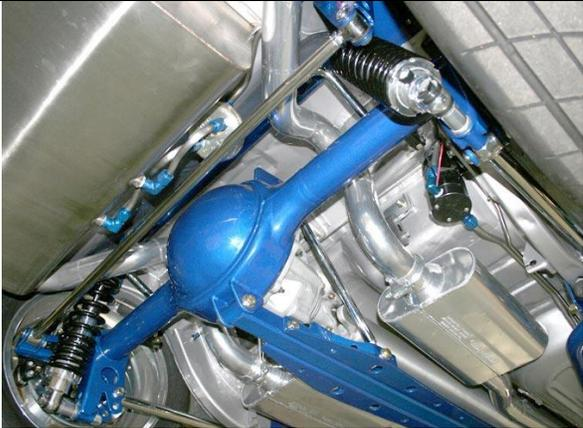
Using a straight edge on the both the housing flanges, measure to the edge of the snubber housings to center housing and adjust panhard bar as needed.
