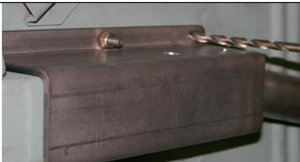
After drilling the first hole, install one of the 5/16 button head bolts through the drilled hole and tighten. This helps in drilling the remaining holes.
