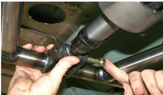
With the heavy lifting done, bolt the front of the Torque Arm slider shaft to the cross member center bracket with the slots using the 1/2 by 3 inch bolt, washers and nut.
