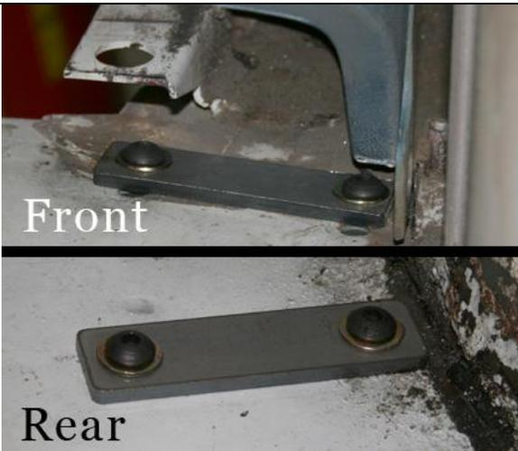
Remove the one alignment bolt and place the slotted reinforcing plate over the inside drilled holes, install the button head bolts and washers through the reinforcing plate, the floor and the outside channel bracket, install nuts and tighten.
