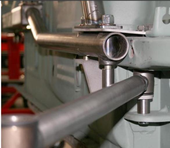
Push the long 6 1/2 inch bolt through the adjuster and brace until it is flush with the brace. Next install the 1 inch long spacer between the brace and stock spring outer flange and finish pushing in the bolt. Install nut and leave loose.
