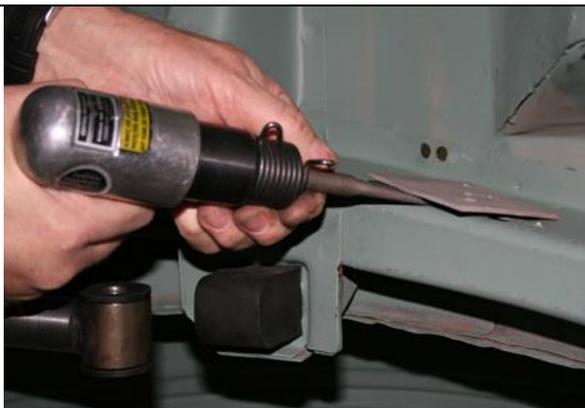
The installation of the coil-over/sway bar mount cross member will require the removal of the two thin stock muffler mounting plates that are spot welded on the inside of each frame rail just behind the axle snubbers. I used a small air chisel to break the spot welds. It left a couple of small holes where the spot welds were but they will be covered up with the channel brackets.
