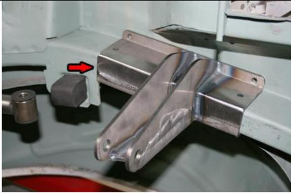
Start with the passenger's side cross member channel bracket with the panard bar bracket welded on. Slide channel over the rail and push forward until the bracket touches the axle snubber flange. See arrow.
