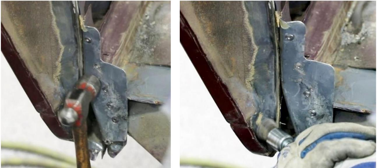
Figure 31 – Adjust Flange
