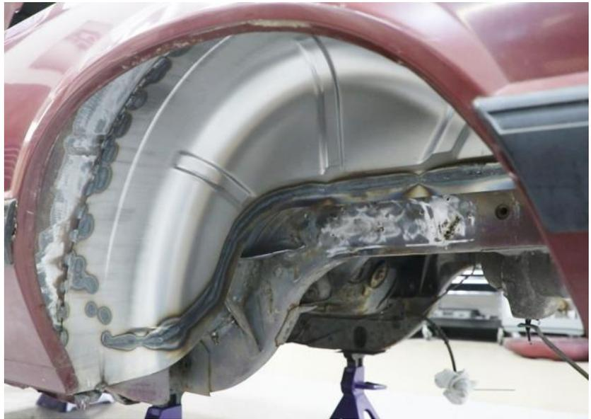
Figure 50 – Mini-Tub Install
