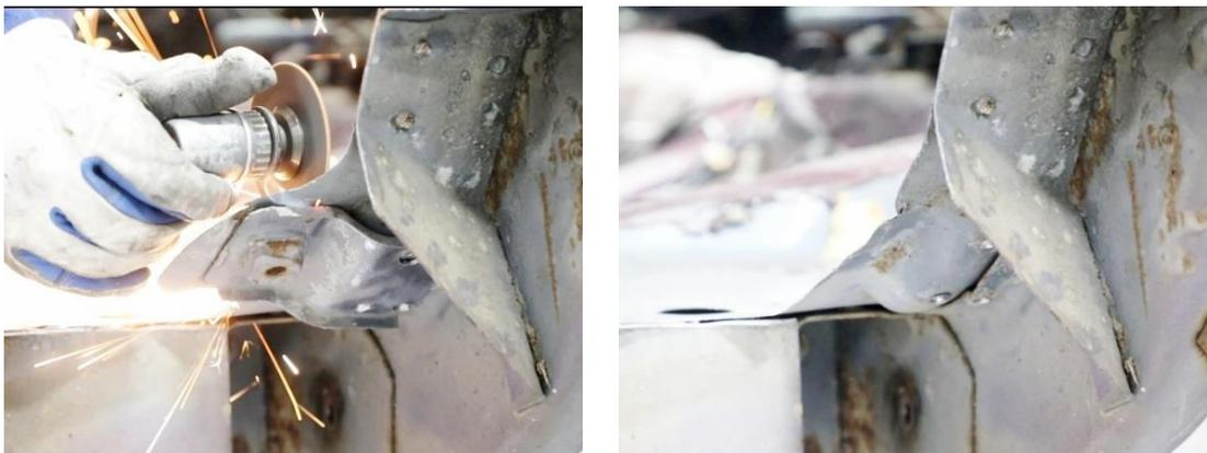
Figure 28 - Remove Seat Belt Anchor
