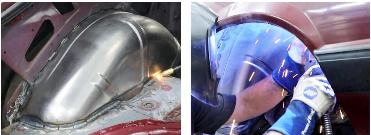
Figure 40 - Finish Weld around Mini-Tub
