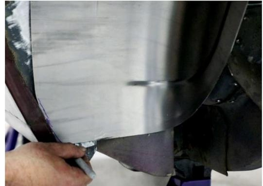
Figure 33 – Test Fit Mini-Tub
