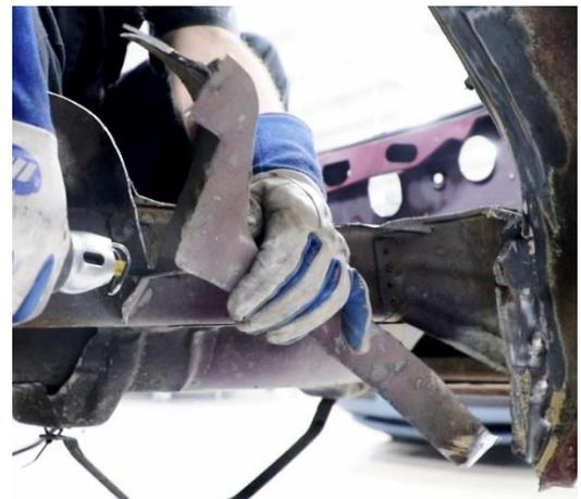
Figure 20 – Remove Rear Factory Structure
