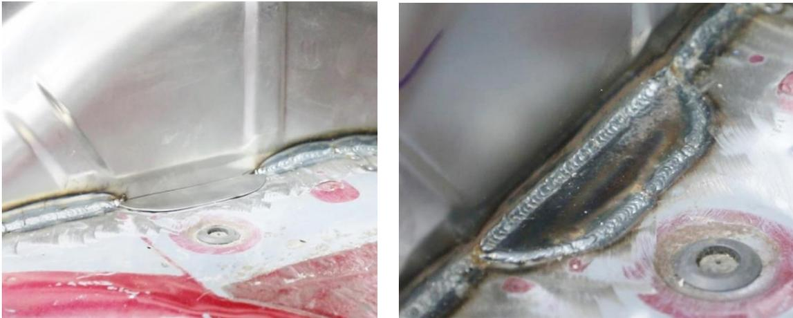
**Figure 42 - Weld Closeout**
