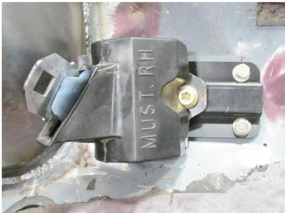
Figure 48 - Torque Seat Belt Assembly
