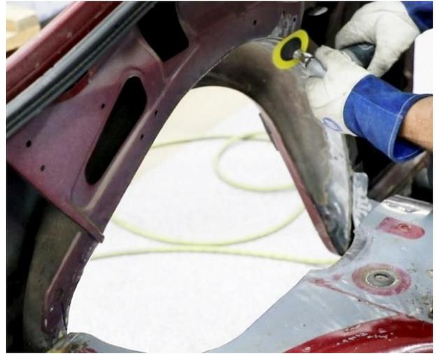
Figure 32 – Grind Sheet Metal
