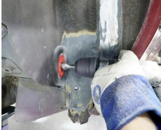
Figure 10 - Locate Spot Welds
