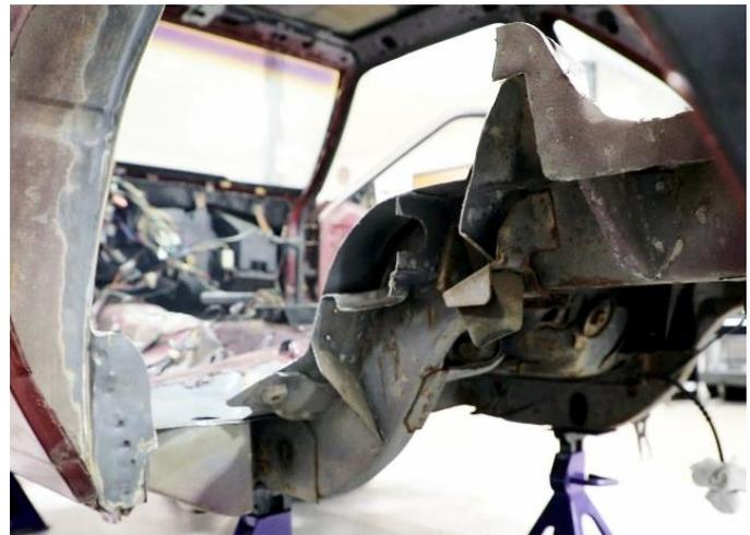
Figure 19 – Remove Front Factory Structure
