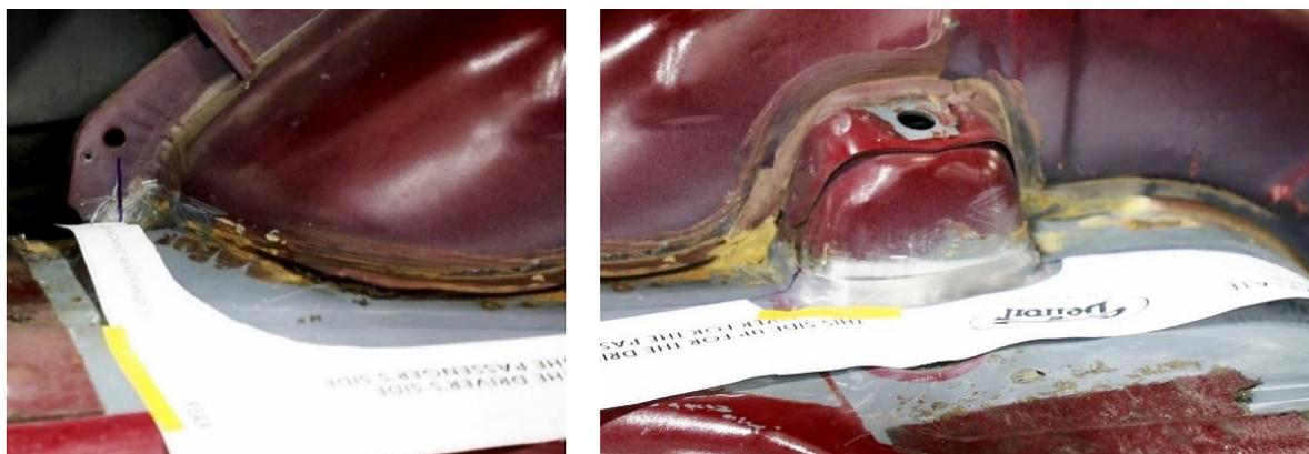
Figure 14 – Locate Rear Template
