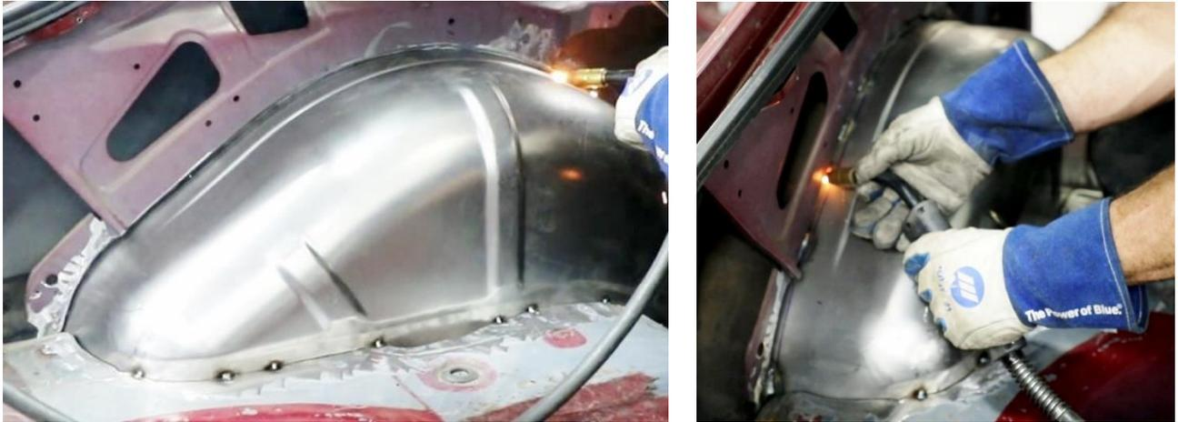
Figure 38 - Tack Weld Mini-Tub
