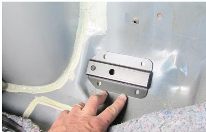
**Figure 43 - Seat Belt Relocation Bracket**
