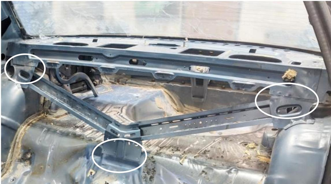
Figure 3 - Remove Wheel Tub Brackets
