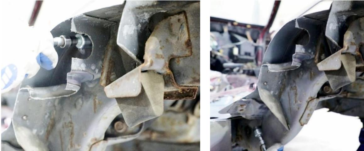
Figure 22 - Expose Spot Welds
