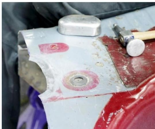
Figure 29 - Flatten Trunk Floor
