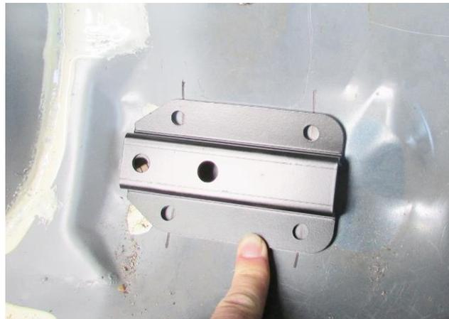
Figure 45 - Transfer Punch Holes
