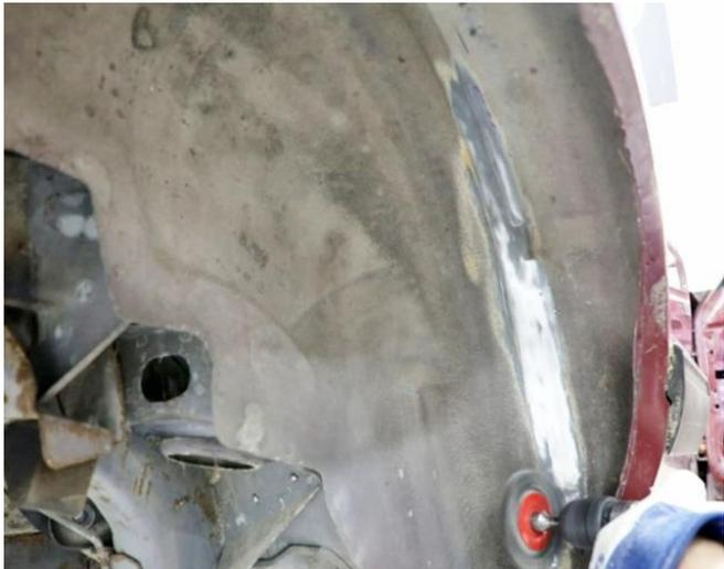
Figure 8 - Remove Undercoating
