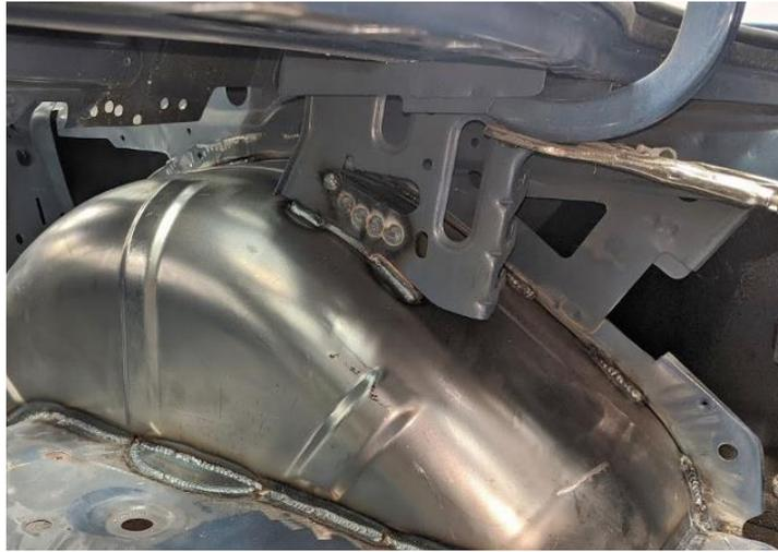
Figure 49 – Re-attach Trunk Hinge Bracket
