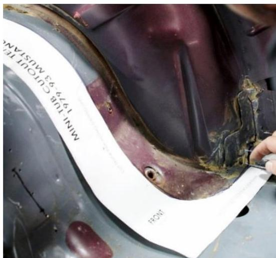
Figure 15 – Locate Front Template
