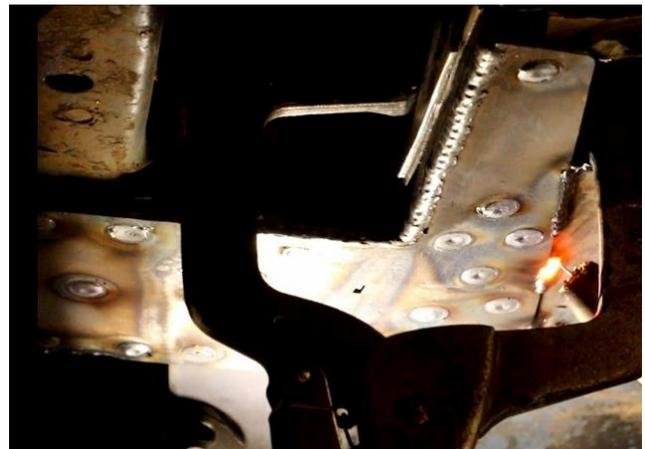
Figure 50 – Plug Weld Torque Box
