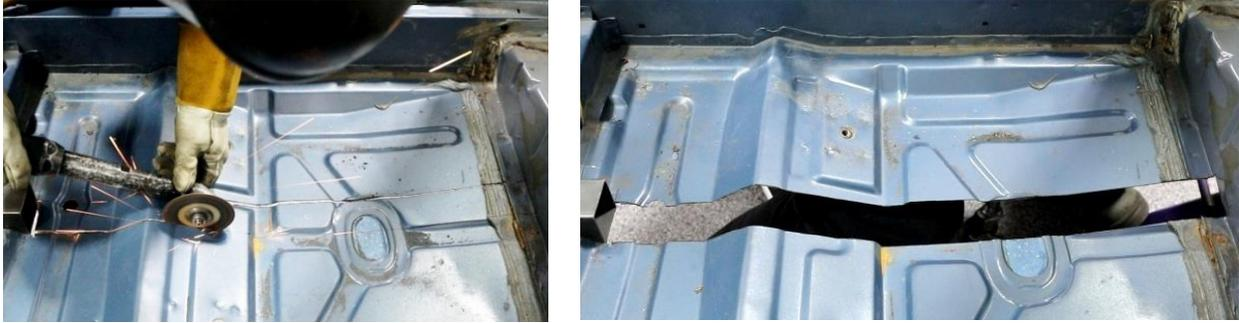
Figure 25 - Cut Floor Pan
