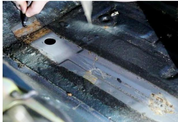
Figure 11 - Mark Front of Cut Area
