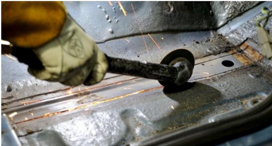
Figure 16 - Cut-Out Floor Section
