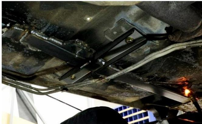
Figure 58 - Finish Weld Rear Connector
