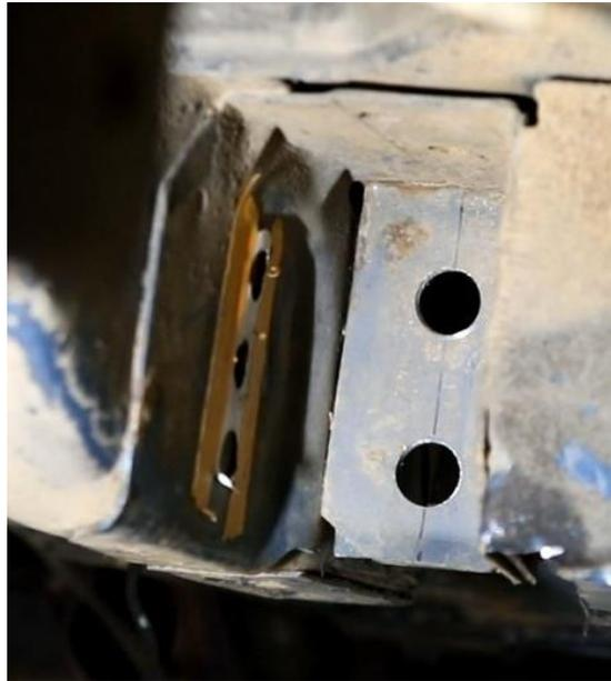
Figure 32 - Drill Plug Weld Holes
