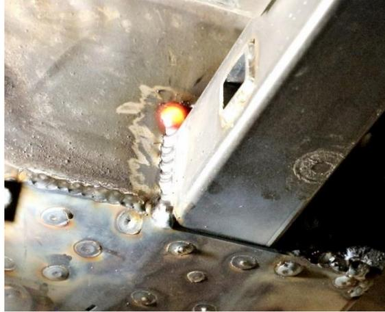
Figure 51 - Weld Rear Connector
