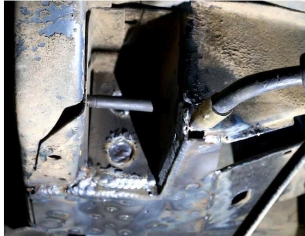
Figure 52 - Weld Link Pocket
