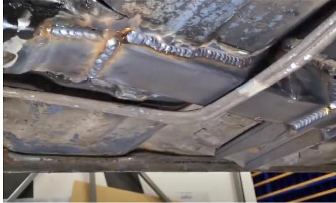
Figure 60 – Secure Fuel Lines
