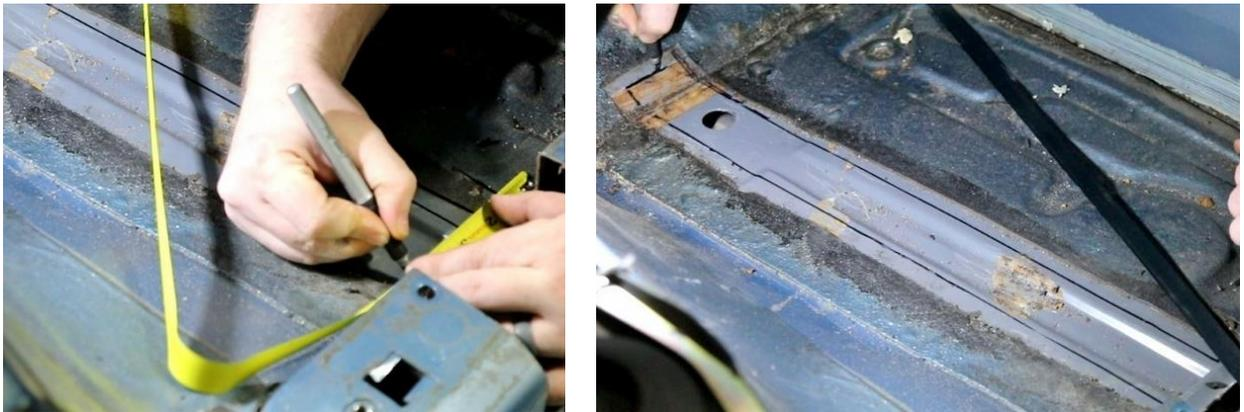
Figure 14 - Mark Inboard Cut Line
