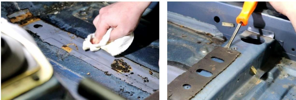
Figure 6 – Clean Cut Area and Remove Foam
