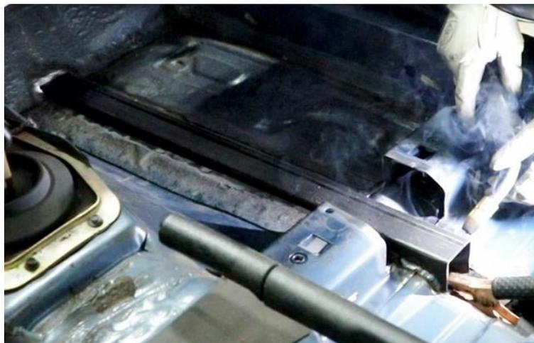
**Figure 43 - Weld Sides of Connector**
