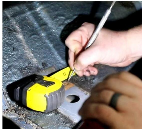
Figure 12 - Locate Cut Line
