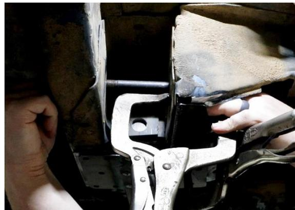
Figure 47 - Position Torque Box Assembly
