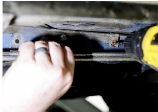
Figure 2 - Remove Fuel & Brake Line Clips
