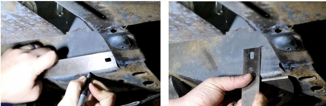
Figure 26 - Locate Lower Link Pocket
