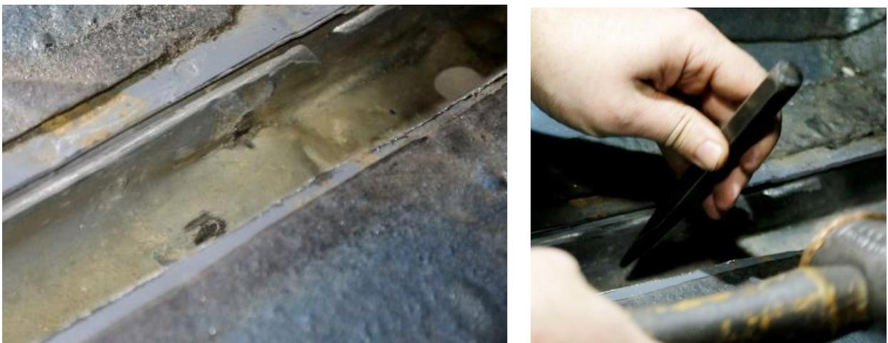
Figure 21 – Grind Away Burrs
