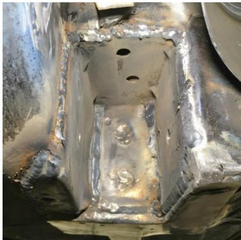
Figure 53 - Weld Factory Sheet Metal
