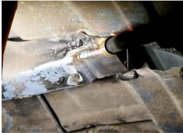
**Figure 42 - Weld Back of Connector**
