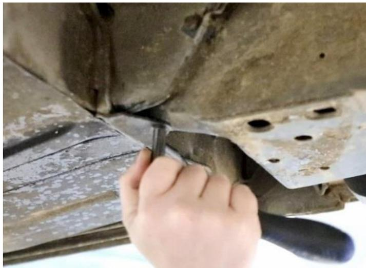
Figure 3 - Remove Brake Line Bracket
