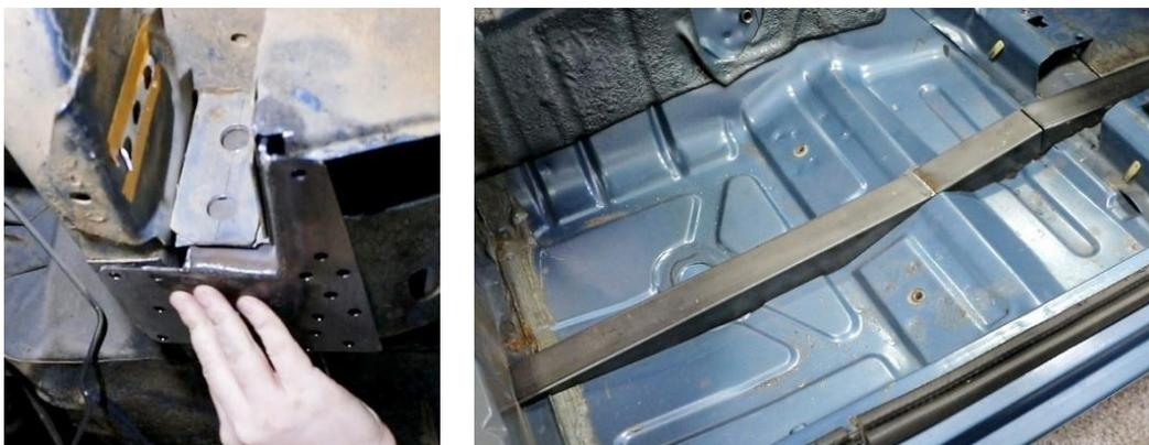
Figure 35 - Clamp Rear Connector Assembly in Place
