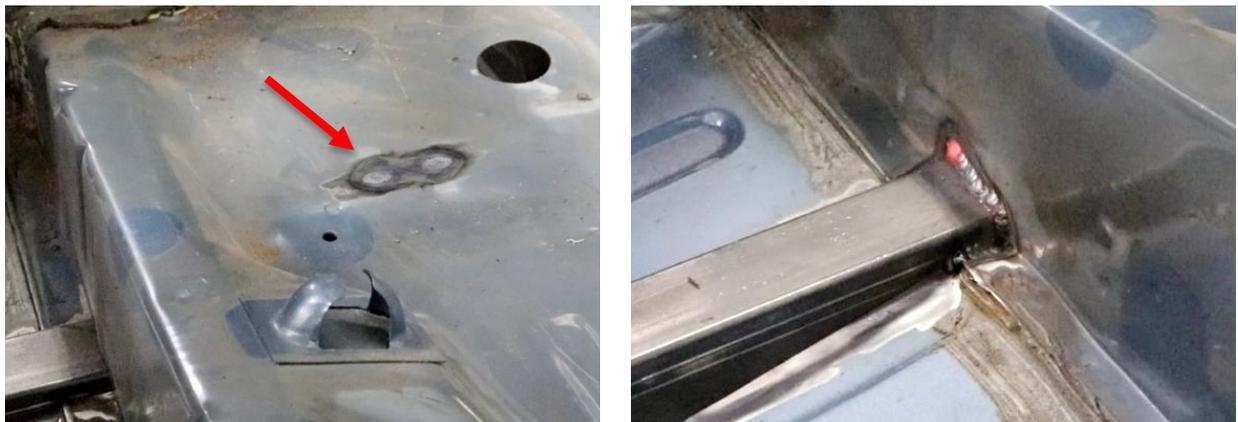
Figure 56 - Weld Seat Riser to Connector
