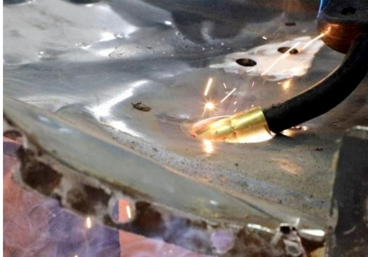
Figure 48 – Tack Weld Torque Box
