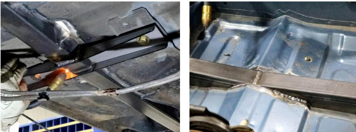
Figure 55 - Weld Seat Mount
