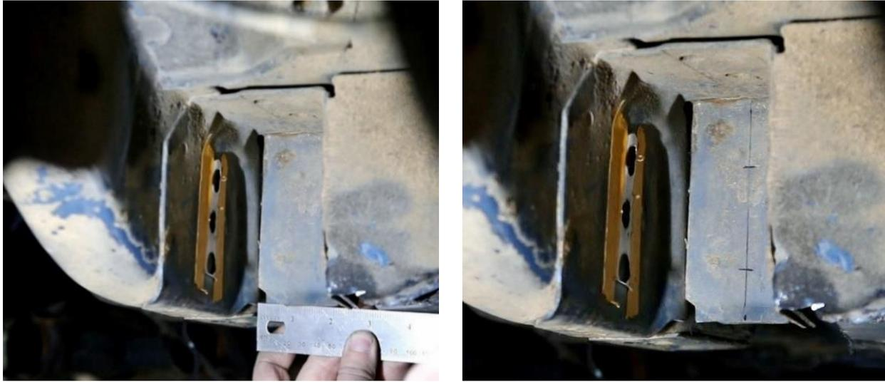
Figure 31 - Locate Plug Weld Holes
