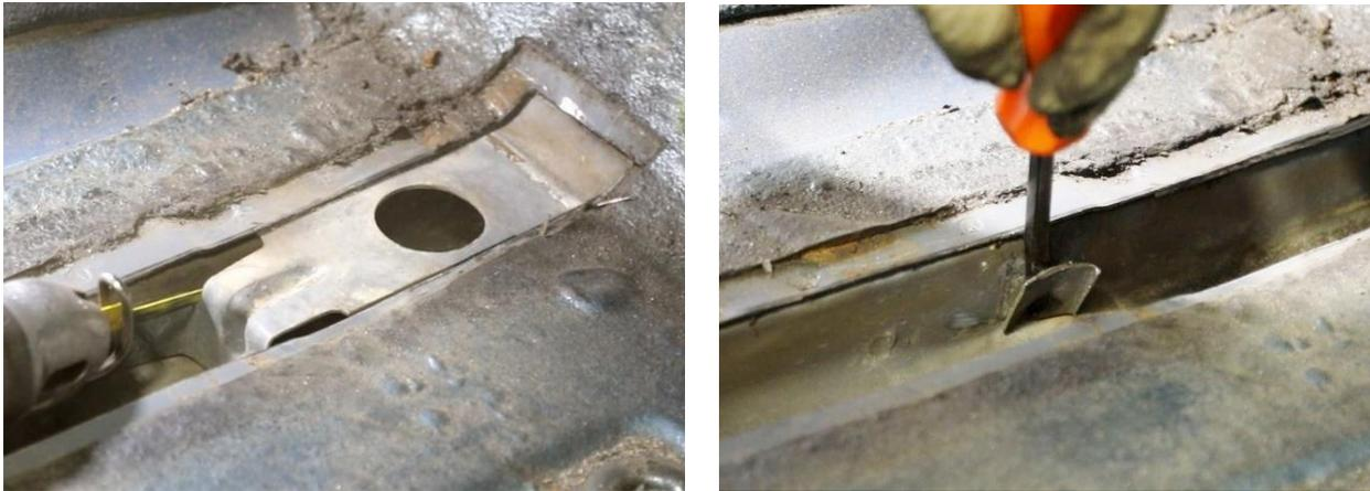
Figure 17 - Remove Floor Pan Bracket
