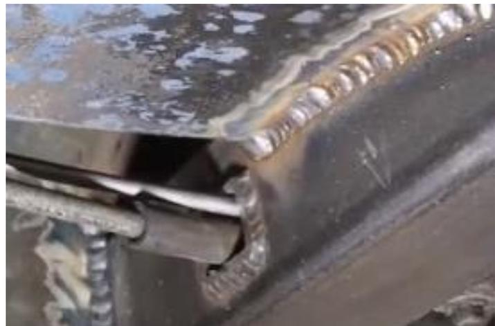
Figure 59 - Secure Brake & Fuel Lines
