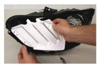
6. Once the epoxy is fully set, reinstall the black panel and white bezel to the main headlight housing using the original screws.
