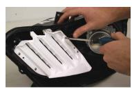
1. Remove the main bezel. Access the factory LED panels by removing the screws holding the DRL housing assembly (white bezel) in place. Once the screws are removed, pull the white bezel away from the headlamp housing.
