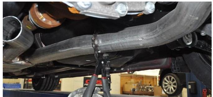
3. Measure 20" away from the flange on the stock resonator, following the outside profile of the exhaust pipe of the passenger side. Using a chain cutter or similar device, cut both the driver and passenger side exhaust pipes at the marked locations. Place a jack stand or similar device under the stock tunnel section of the exhaust for support. **WARNING:** Once the axle pipes are cut, there are no additional stock hangers supporting the tunnel section.
