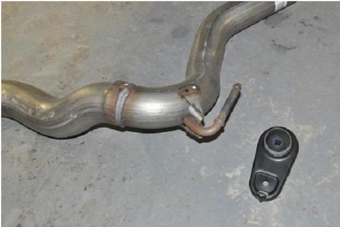
5. Remove both the driver and passenger side hanger grommet assemblies from the front muffler hangers using grommet pullers or a similar device. **Save both grommets for reinstallation** (Install Step 4).
