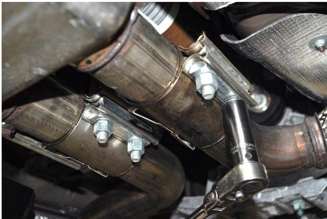
2. Using a 3/8" drive ratchet and 15mm deep socket, loosen the two sleeve clamps at the cat-back connection point. Both nuts must be loosened in order for the clamp to fully disengage.
