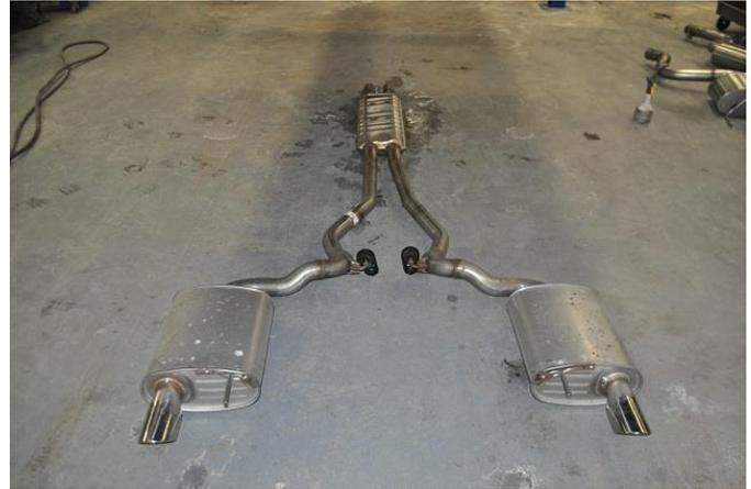
4. Slide the stock exhaust assembly rearward until the stock resonator inlet pipes are free of the sleeve clamps. Lower the front of the exhaust in order to create clearance between the resonator inlet pipes and the sleeve clamps, then slide the complete exhaust forwards to remove the rear driver and passenger side hangers from their respective hanger grommets. The stock exhaust assembly will now be free from the vehicle.
