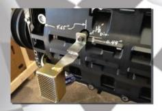
Image left shows the location you will need to modify the tray in order to properly mount the pickup tube. In addition to this modification you will also need to move the pickup mounting bolt from the OE position to this location.
