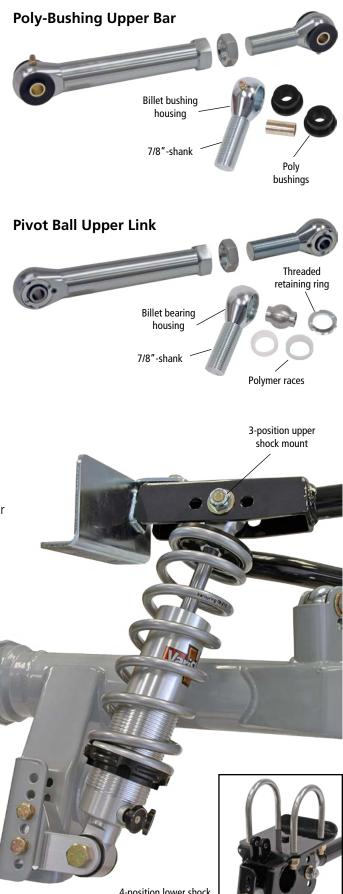
4-position lower shock mount standard on both FAB9<sup>™</sup> welded bracket and bolt-on leaf-spring housing bracket
