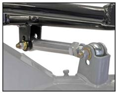
2-position chassis and housing arm brackets
