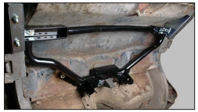
"Self-positioning" system uses existing pinion snubber and top shock mount bolt holes.
