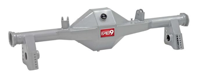
Engineered to accept all 9", Ford-style differentials, each FAB9™ includes a fully-welded center section with internal gussets, 3" axle tubes, and Ford big-bearing, late-model Torino, housing ends. All housings are manufactured in-house utilizing our state-of-the-art robotic spray-arc welder. Weld penetration, and quality are absolutely outstanding, guaranteeing consistent, reliable performance. Center
