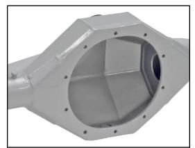
Robotic spray-arc welded center section with internal tube gussets
