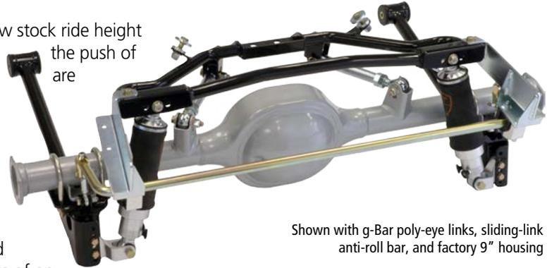
Shown with g-Bar poly-eye links, sliding-link anti-roll bar, and factory 9" housing
