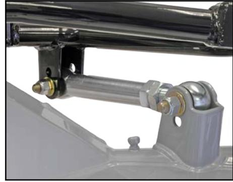
2-position chassis and housing arm brackets
