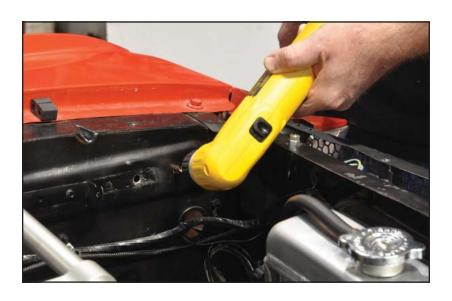
10. Secure the reservoir to the inner fender with the 5/16-18 x 1/2" button heads and flat washers supplied with the adapter.
