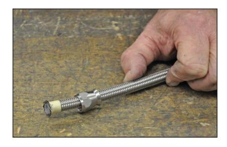
19. Place the brass ferrule in between the Teflon hose and steel braid as shown.
