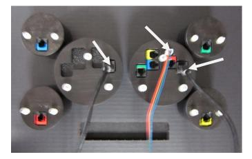
3. Connect the provided CAT5 Cables and the switch harness to the back of the Speed and Tach if applicable and carefully route the other ends to the control box mounting location.
