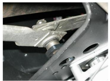
Figure 6 - Attach Wiper Linkage to Pitman Arm
