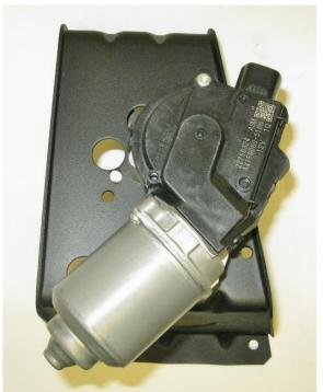
Figure 4 - Wiper Motor
