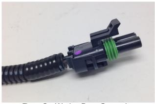
Figure 9 - Washer Pump Connection
