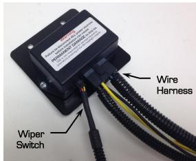
Figure 10 - Connect Wiper Switch & Harness to Module
