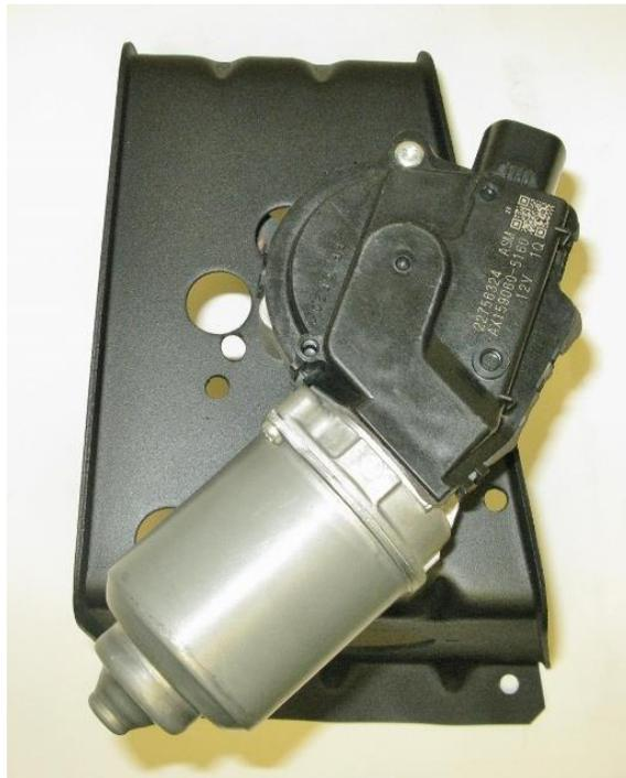
Figure 4 – Wiper Motor
