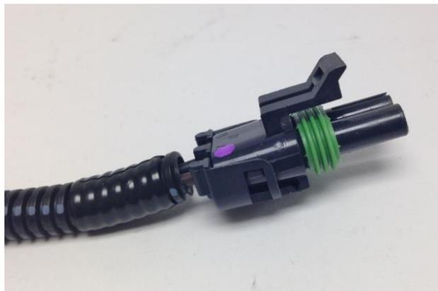
Figure 9 - Washer Pump Connection
