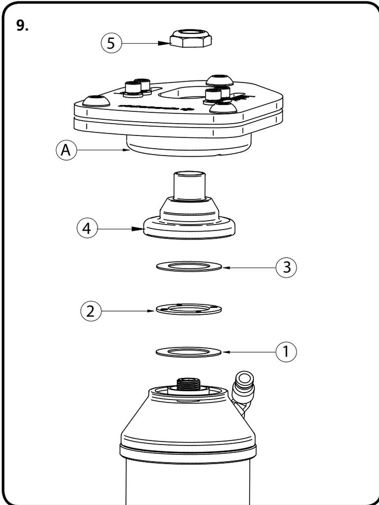
9. Install the Air fitting into the Airspring using thread tape. The Strut comes preassembled, but if for some reason you need to disassemble the strut, Figure 9 shows the assemble order. Remove the Adjuster Knob from the Strut shaft for assembly. Bolt the strut assembly into the upper mount (A), see diagram 9 for assembly order.
