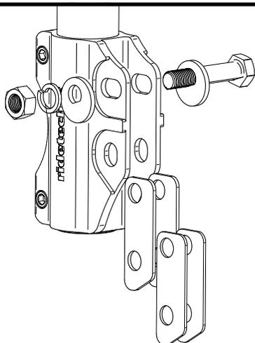
**10.** Due to various thickness of the spindles, the kit comes with shims for the spindle. It may necessary to run multiple shims of some. If multiple shims are required, install (1) Thick and (1) Thin on each side of the spindle. The lower Strut mounting holes reuses the OEM Bolt. The upper Slotted holes use the 16mm Eccentric Bolt provided in the kit. This Eccentric Bolt is used for camber adjustment.
