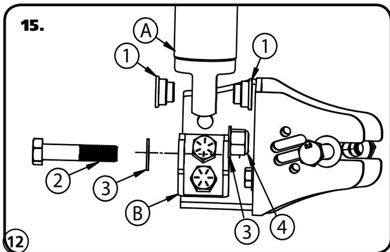
**15. 16.** Install the ShockWave(A) in the Lower Shock Mount(B) using a 90002043 Spacer(2) inserted into each side of the Shock bearing. Slide the shock into the stock mounting location. It may be necessary to use the jack and raise the differential to align the mounting holes. With the mounting holes aligned, insert a 1/2"-13 x 2 1/2" Bolt (3) and 1/2" Washer (4) through the Mount and Shock. Install a 1/2" Flat Washer (4) and 1/2"-13 Nylok Nut (5) on the Bolt and Tighten.
