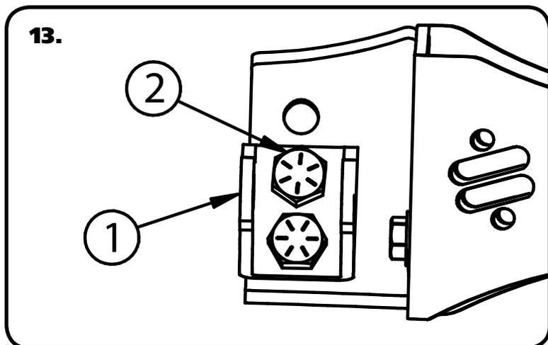
**13.** Attach the 2 Hole Lower Shock Mount(1) to the Main Mount using 1/2" x 1" bolts (2) with a Flat Washer and Nylok nut on the back side. The Mount bolts to the 2 lower holes. If a higher ride height is desired, the top 2 holes can be used.
