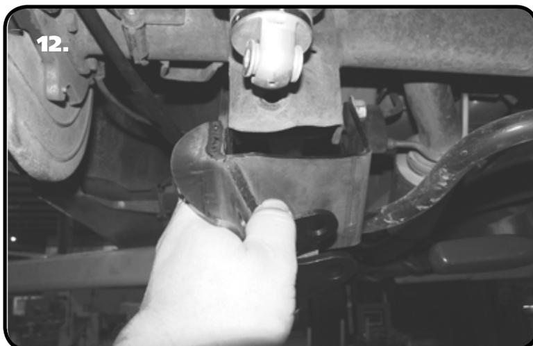
**12.** Slide the Lower Shock mount on to the Axle Mount. The Shock Mount wraps around the OEM Control Arm mount. The Slots on the side of the Mount slide on the Lower Control Arm Mounting Bolt. Install (1) 3/8-16 x 1 1/4" bolt (Threads pointing forward) through the hole in the Shock Mount and Lower Control Arm Mount. Install a 3/8" Flat Washer and 3/8" Nylok Nut on the Bolt and tighten. Tighten the Lower Control Arm Bolt.
