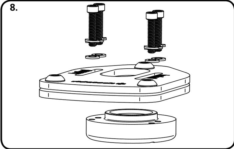
8. Attach the Bearing Housing to the Caster Plate Assembly. The Housing is positioned with the 4 threaded bolt holes to the front of the car lining 2 holes up with each slot. Insert the housing up from the bottom. Apply Antiseize to the threads of each of the (4) 1/4" x 1 1/4" Socket Head Bolts. Install a 1/4" Lock Washer and Flat Washer on each bolt. The bolts will be inserted through the caster plate with 2 bolts in each slot threading into the Bearing Housing.
