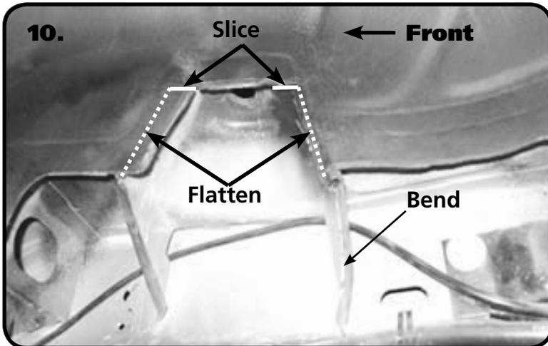
**10.** Illustration 10 shows the modifications that need to be done to the Shock opening for Shock-Wave clearance. The rear has been done in the picture to show what the end result should look like. Slice the sheetmetal at the top of the opening forward and backward even with the top of the opening. With the sheetmetal sliced, bend the pinch weld inward until it is flat against the front and back of the opening. Bend the rear brace back to clear the Air Spring on the Shockwave.
