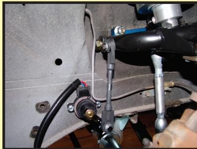
5- Once both sides of the linkage have been finished, secure the linkage to the sensor and suspension.
