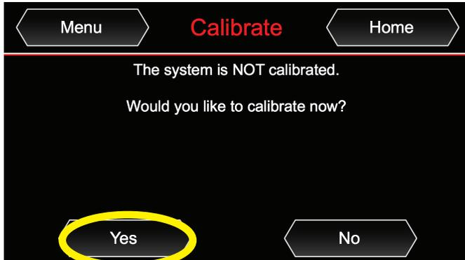
Make sure nothing is under the vehicle before performing calibration. To Calibrate the system, select "Yes".
