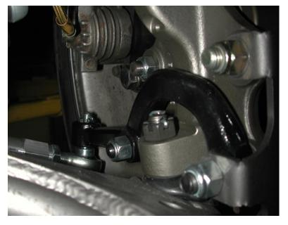
12. Slide the ball joint boot over the ball joint, then place the spindle over the ball joint stud. A ball joint spacer will be necessary to align the castle nut with the cotter pin hole. Grease ball joint
