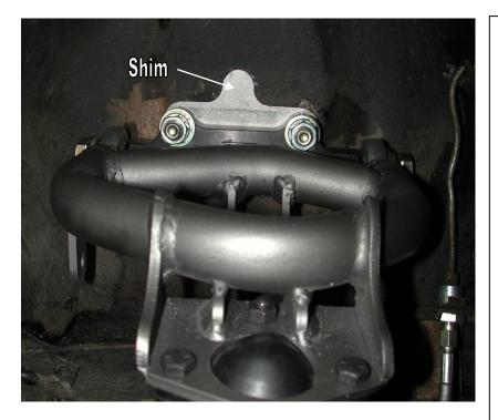
**2.** Bolt the upper StrongArm to the body using  $\frac{1}{2}$ " x 2  $\frac{1}{2}$ " bolts, flat washers and lock washers. The **ARROW** points to the front of the vehicle. A shim is supplied and may need to be installed between the body and the arms to achieve proper alignment.
