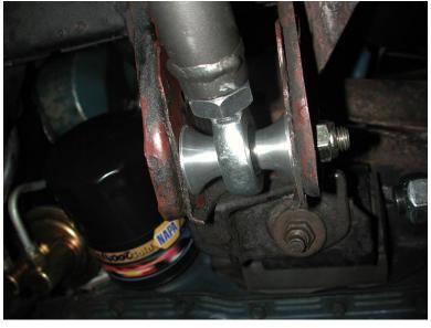
8. The bearing stud should already be threaded into the lower arm, factory set at 2-7/8" (measuring from the end of the arm to the bearing).
