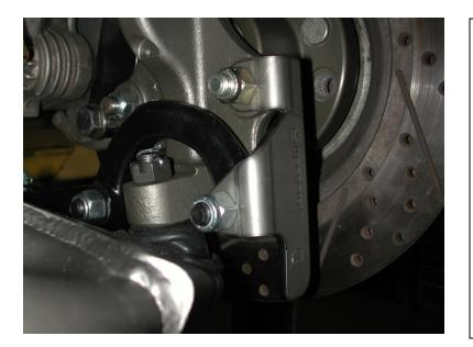
3. Install the Ridetech spindle on the control arms.
