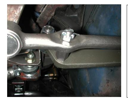
2. The studs with the long hex on them will get installed into the factory draglink with the taper going into the draglink, a 7/16" castle nut is used to attach it to the draglink. Torque the nuts to 35 ft lbs and tighten as needed to align cotter pin hole and install cotter pin. The straight shank will point to the front of the car.
