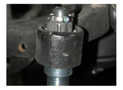
5. Install the stud with the round flange into the steering arm with the taper going into the steering arm. Torque the nuts to 35 ft lbs and tighten as needed to align cotter pin hole and install cotter pin.
