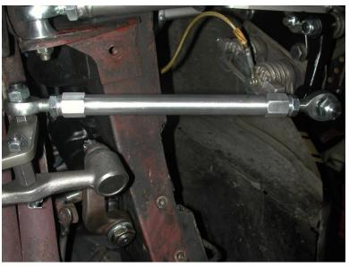
7. The tie rod can now be assembled to a center to center length of 14 ¼" to start with having equal amount of threads on both ends. These Aluminum adjusters have a left hand thread on one end and a right hand thread on the other. You should use anti seize when threading the heim ends into the adjuster.
