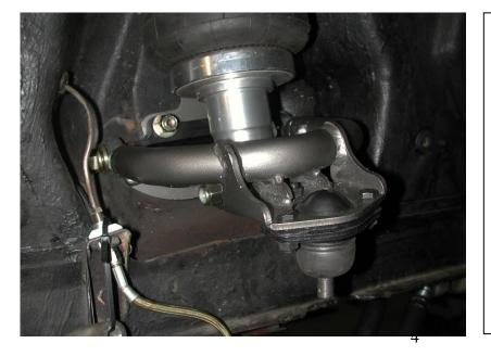
**4.** Bolt the upper arm to the spindle using the hardware and cotter pin supplied.
