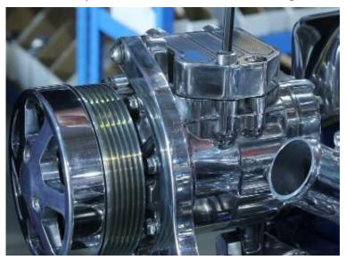
3. Install the compressor manifold using 2) M8 X 1.25 X 25mm socket cap screws. Apply anti-seize to the threads and tighten fully while using caution to prevent over tightening. **WARNING! Do not connect power to the AC clutch wire without first connecting hoses and fully charging your air conditioning system. Please follow all of the enclosed instructions for charging your system. Use of improper charging methods could cause serious damage to your compressor that will not be warrantied.**
