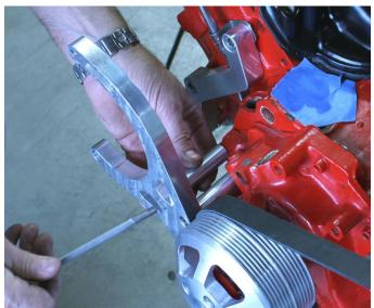
1. Coat the threads of 1) 5/16-18 X 4-3/4" socket cap screw with RTV sealer and insert into hole A on the air compressor bracket. Use 1) 2-5/8" spacer on the bolt, behind the bracket, and thread into the block. Repeat with 1) 5/16-18 X 4-1/2" socket cap screw and 1-1/2" spacer in hole B and 1) 5/16-18 X 4-1/2" socket cap screw and 2-5/8" spacer in hole C. Tighten equally and completely. Use caution so as not to over tighten.
