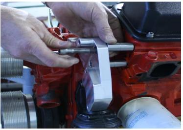
1. Using 4) 1-3/4" spacers between the bracket and the block, attach the bracket using 4) 7/16-14 X 2-1/2" socket caps screws. Coat all stainless steel fasteners liberally with anti-seize and tighten thoroughly.
