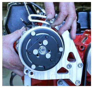
2. Use 2) 8MM-1.25 X 30MM button head bolts to attach the compressor to the top and bottom of the mounting plate. Use anti-seize on the threads but do not fully tighten at this point.
