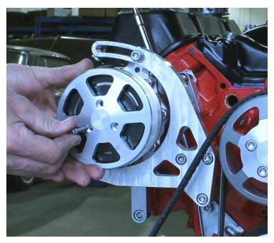
4. Apply Loctite to 3)  $1/4-20 \times 3/4$ " socket cap screws and use to install the air compressor cover onto the compressor. Tighten fully while using caution to prevent over torqueing.
