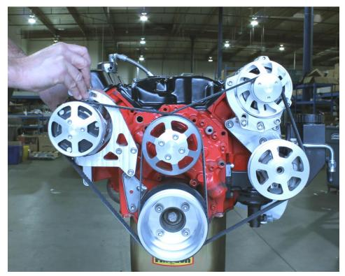
4. Install belt #K0604311 around the water pump, crank, and air compressor pulleys.
