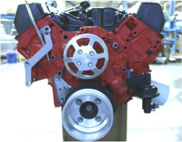
1. Use 4) 3/8-24 X 1" socket cap screws and 4) beveled Bellville washers to attach the crank pulley. Make sure that it seats completely in the recess on the balancer. Coat all stainless steel fasteners liberally with anti-seize and tighten thoroughly.
