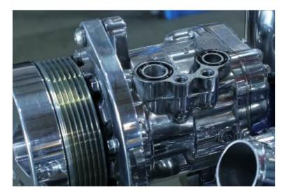
2. With the plate removed, you will see the two sealing o-rings. Leave these on the compressor and be careful not to damage them.
