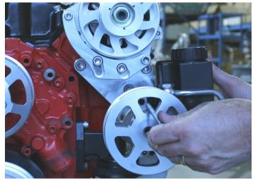
1. If you are using a power steering pump with an attached reservoir, install the hardline into the pump. Do not tighten as you will need to remove it once you have measured for your power steering line length. 2. Use 2) 5/16-18 X 3" socket caps screws and 5/16 lock washers to fasten the power steering pump to the bracket. Remember to apply antiseize to the threads and tighten thoroughly.
