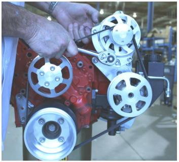
1. Install belt #K060478 around the water pump, crank, power steering and alternator pulleys.
