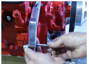
2. Using 1)  $3/8-16 \times 1-3/4''$  socket cap screw and 1) .670'' long spacer, attach the bottom of the bracket to the block. Do not tighten at this point. Use 1)  $7/16-14 \times 1''$  socket cap screw to fasten the top of the bracket to the cylinder head. Tighten both bolts completely
