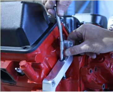
1. If present, remove your dipstick and tube and slide it through the hole in the bracket.
