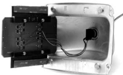
13. Remove the backing from the tape on the LED assembly and insert assembly into the tail light housing keeping the assembly centered in housing. Make sure the arrow is still pointing up. Press firmly on the bracket to ensure good tape bonding.
