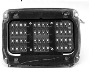
15. Test the tail lights, brake lights, and turn signals. If the turn signals do not flash you will need to upgrade your flasher. If you are replacing only the rear turn signals you should be able to use a heavy duty electronic flasher from your local parts store. If you are replacing both front and rear or do not have front bulbs you will need a no-load flasher, Dakota Digital part number LAT-NLF.
