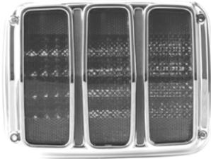
1. Remove both right and left tail light lenses as described below at the same time, taking care to keep the left and right lenses and trim with the correct side of the vehicle.
