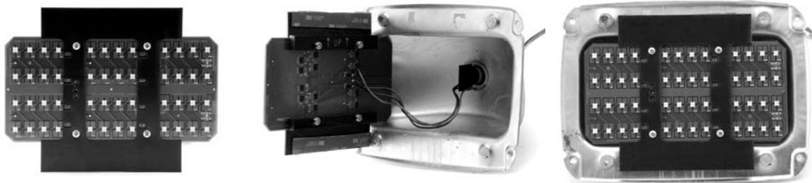
9. Squeeze the primer tube to break the glass bulb and wet the brush end with primer. Rub the primer on the lenses and the housings at the places where the tape will touch. Treat both left and right housings and lenses at the same time before the primer tube dries out.
