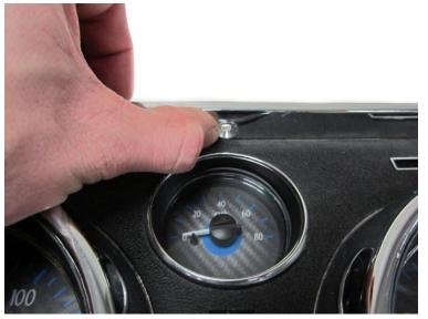
11. Use the three (3) aluminum spacers and 7/8" flat head screws from the hardware pack to secure the top portion of the bezel to the dash. From the front of the bezel, press in the spacer followed by the flat head screw to secure it in place. Note: some reproduction bezels may require sanding a flat edge on the outer most diameter to fit inside the hole.
