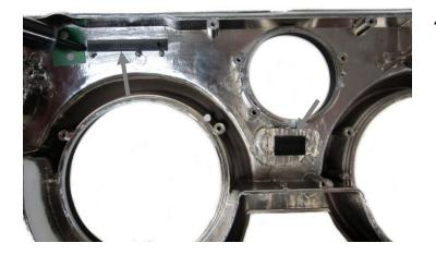
4. The stock indicators for Brake and High Beam will not be used. Two, small, block-off plates are included; these carry engraved part numbers, 636108 and 636109, for Brake and High Beam respectively. RTV silicone works well to secure these plates. Be sure to glue the pieces with the textured side down to ensure the part numbers are not visible from the front side.
