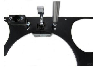
7. Mount the Wiper switch to the ABS plastic panel with the smooth side facing you. The Wiper switch will fit into the large cross hair, and the arm of the switch will slide through the ABS from the rear. Use the provided 3/8" screws with lock washers and nuts to mount the wiper switch to the panel.
