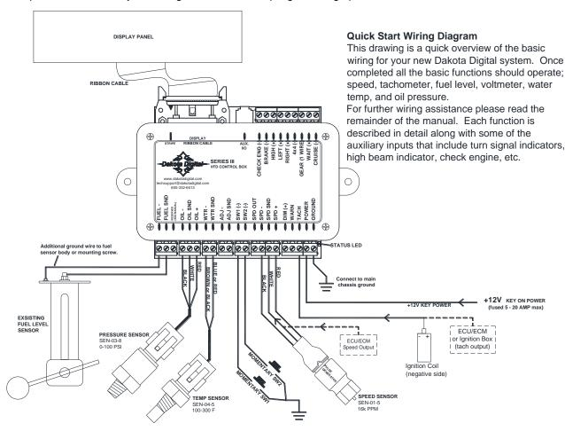
• Set up the control box to match your vehicle. The tachometer must be set to match the number of engine cylinders and the fuel gauge must be set to match your fuel sender resistance curve or the instrument system will not display correctly. The control box can read seven common fuel level sender resistance values. If your sender is not listed, the system can be programmed to a custom sender (see full manual for details).
