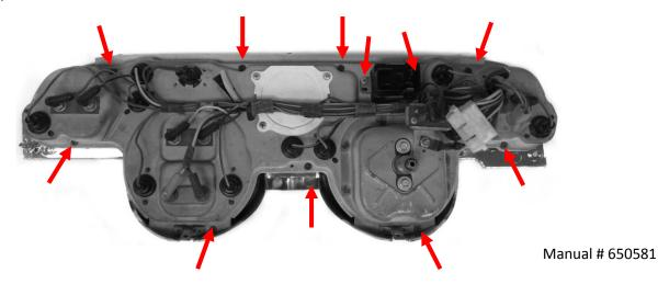
2. Remove the stock gauges, separator plates, and lenses from the bezel.
