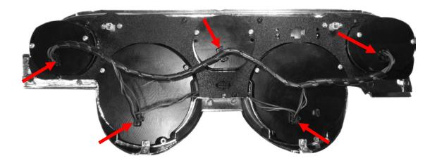
11. This system comes with the option to use two sets of turn signals in your dash: arrows located in the faceplate of your new HDX display, and arrows in your vehicle's stock turn signal locations. To use the new faceplate arrows, follow the wiring instructions for the turn signals found in the main HDX manual.
