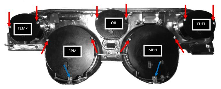
6. The cluster should look as shown starting from the left FUEL, MPH, OIL, RPM, TEMP.
