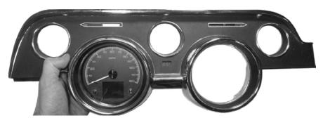
5b. Use the provided 2" screws to mount the gauges in place. Do not fully tighten; the holes are slotted to allow minor adjustments to perfectly align each gauge. For the Speedometer and Tachometer, use the two provided brackets at the bottom slots as shown in blue arrows. Once aligned, finish tightening the 12 screws.
