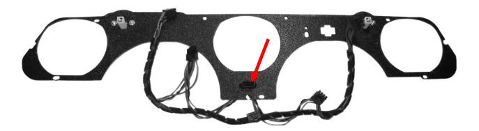
9. Lay the ABS panel over the back of the gauge cluster with the smooth side down and slip the wiper arm through the appropriate opening in the bezel. Use the seven (7) supplied ½" black screws to mount the panel to the back of the bezel. Ensure harness wires are not pinched.
