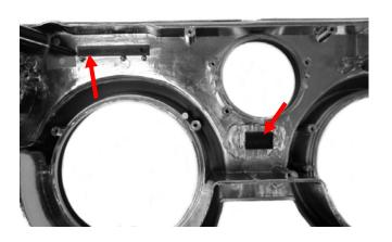
4. The stock indicators for Brake and High Beam will not be used. Two, small, block-off plates are included; these carry engraved part numbers, 636108 and 636109, for Brake and High Beam respectively. RTV silicone works well to secure these plates. Be sure to glue the pieces with the textured side down to ensure the part numbers are not visible from the front side.
