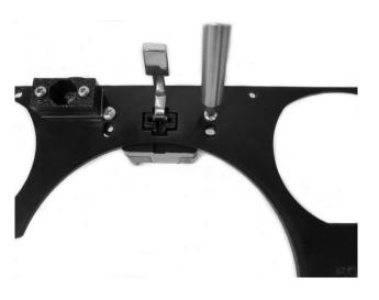
7. Mount the wiper switch to the ABS plastic panel with the smooth side facing you. The wiper switch will fit into the large cross hair, and the arm of the switch will slide through the ABS from the rear. Use the provided 3/8" screws and nuts to mount the wiper switch to the panel.
