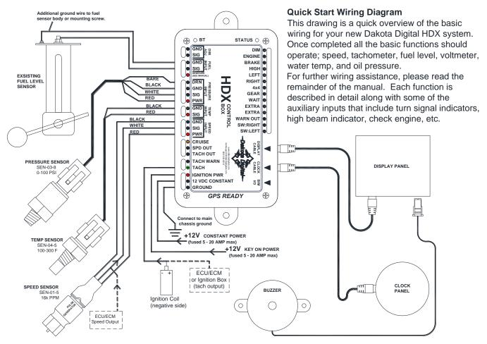
• Set up the control box to match your vehicle. The tachometer must be set to match the number of engine cylinders and the fuel gauge must be set to match your fuel sender resistance curve or the instrument system will not display correctly. The control box can read 10 common fuel level sender resistance values. If your sender is not listed, the system can be programmed to a user settable sender (see full manual for details).
