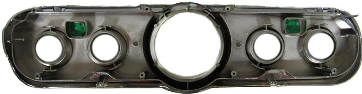
3a. Remove the protective tape from the clear lens and install the VHX system into the bezel. Watch carefully as you insert the system so you don't scratch or damage the lens.
