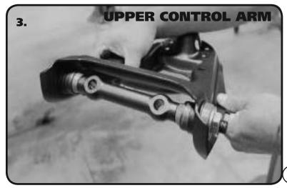
2. Disassemble the Bushing being installed. When installing Bushings in the control arms, insert the Cross Shaft before installing any Bushings. Support the back side of the flange the Bushing is being Installed in. They can be supported by either the piece of Metal or by the Bench Vise with the Jaws opened wide enough to let the Bushing Shell pass through (Figure 2).
