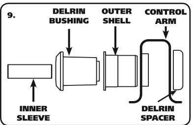
**9.** Install the Outer Shell into the control arm. Next, install the Delrin Bushing into the Outer Shell followed by the Inner Sleeve. With the Delrin Bushing and Inner Sleeve installed, install the Delrin Spacer over the SMALL end of the Delrin Bushing. The ROUNDED surface will be out, away from the control arm.
