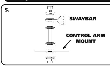
5. Install the End Links. Use (Figure 5) for proper installation. Tighten the Hex Nut enough to slightly compress the Bushings.
