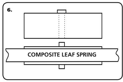
**6.** This Kit use a Lowering Block to help get the proper design height. Install the 1 1/2" Lowering Block on top of the leaf spring with the locating pin inserted into the center hole of the block. Lower the differential with the Lowering Block in place like shown in (Figure 6). The PIN on the Lowering Block needs to be inserted into the HOLE in the OEM leaf spring mount.
