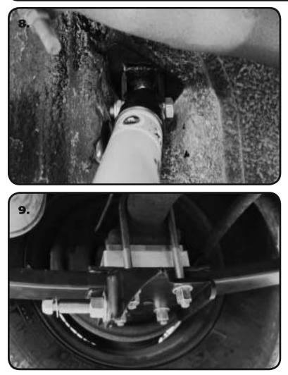
**8.** The Shock is mounted in the Upper Mount with the BODY UP. It is held in place with a  $1/2"-20 \times 2 \ 1/4"$  Hex Bolt & 1/2"-20 Nylok with a 1/2" Flat Washer on each side of the bracket.
