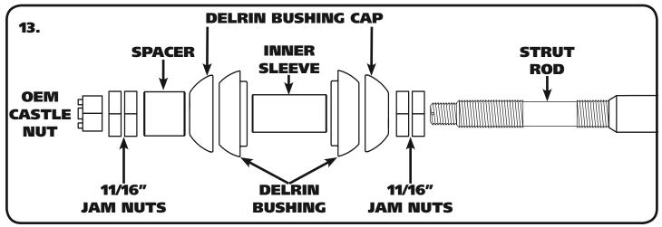
**13**. Install (2) 11/16" Jam Nuts on the INNER THREADS of the strut rod followed by the Delrin Bushing Cap. Insert the strut rod through the Bushing Sleeve until the Ball is nested into the Bushing Cap. Install a second Bushing Cap on the strut rod followed by the Spacer. Next, install the (2) 11/16" Jam Nuts on the OUTER THREADS. Install the OEM castle nut on the end of the strut rod with a cotter pin through it. Position isn't critical, it will be adjusted when the front end is aligned.
