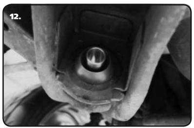
**12.** Install the Inner Sleeve in the Strut Rod Bushings. Center the Sleeve in the Bushings, this will also help hold the Bushings in place during reassembly of the strut rod.
