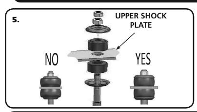
5. Install a Stud Top Bushing & Bushing Washer on the Shock. Install a 3/8"-24 Jam nut on the threads and tighten until the Bushings just start to bulge. Install a 2nd 3/8"-24 Jam Nut and tighten it against the 1st.
