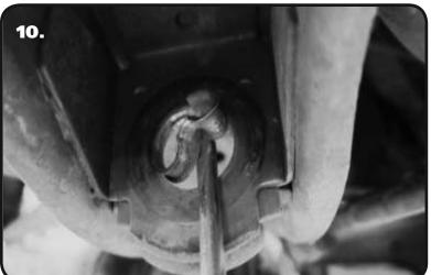
**10.** A Delrin Bushing setup for the strut rod is also included in this kit. The liner that is installed in the frame hole has to be removed. Use a chisel to distort it and remove it. In **(Figure 10)** we distorted it from the bottom edge and removed it.
