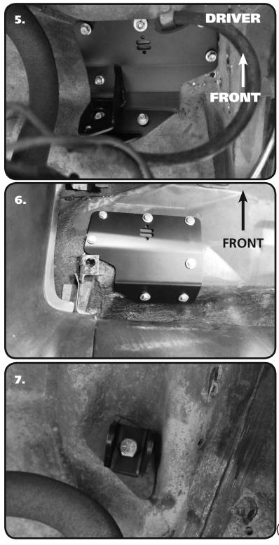
**5.** The Driver Upper Shock Mount repositions the top of the shock behind the axle. The Mount nests in the car one way. Position the Mount in the car with the Shock attaching point to the rear and away from the frame. The outside edge of the mount will touch the frame with the front edge against a body seam. Using these points as a guide, the Mount will fit the contours of the body. With the Mount in position, use it to mark the 7 holes and drill them 5/16"
