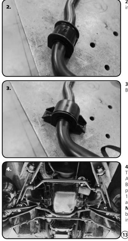
**2.** Open up the Poly SwayBar Bushings and install them over the Delrin Sleeves.
