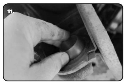
**11.** Refer to **(Figure 13)** for the Delrin Strut Rod Bushing assembly order. The Delrin Strut Rod Bushing will insert into the frame bushing hole with the rounded side of the bushing outward. A Bushing needs to be installed on both the front and rear side of the frame.
