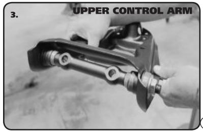
2. Disassemble the Bushing being installed. When installing Bushings in the control arms, insert the Cross Shaft before installing any Bushings. Support the back side of the flange the Bushing is being Installed in. They can be supported by either the piece of Metal or by the Bench Vise with the Jaws opened wide enough to let the Bushing Shell pass through (Figure 2).
