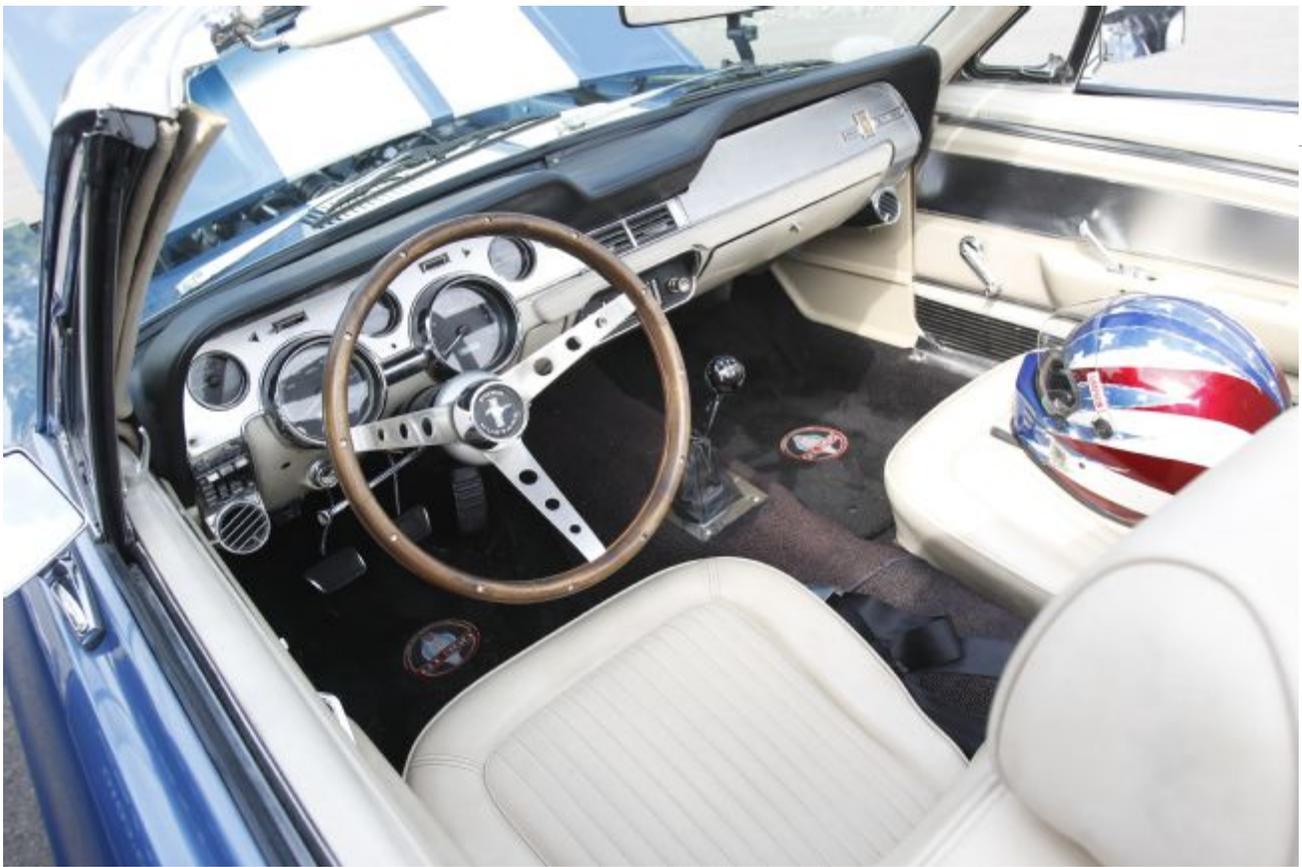
**A factory steering wheel hides the Dakota Digital speedo and tachometer.**
