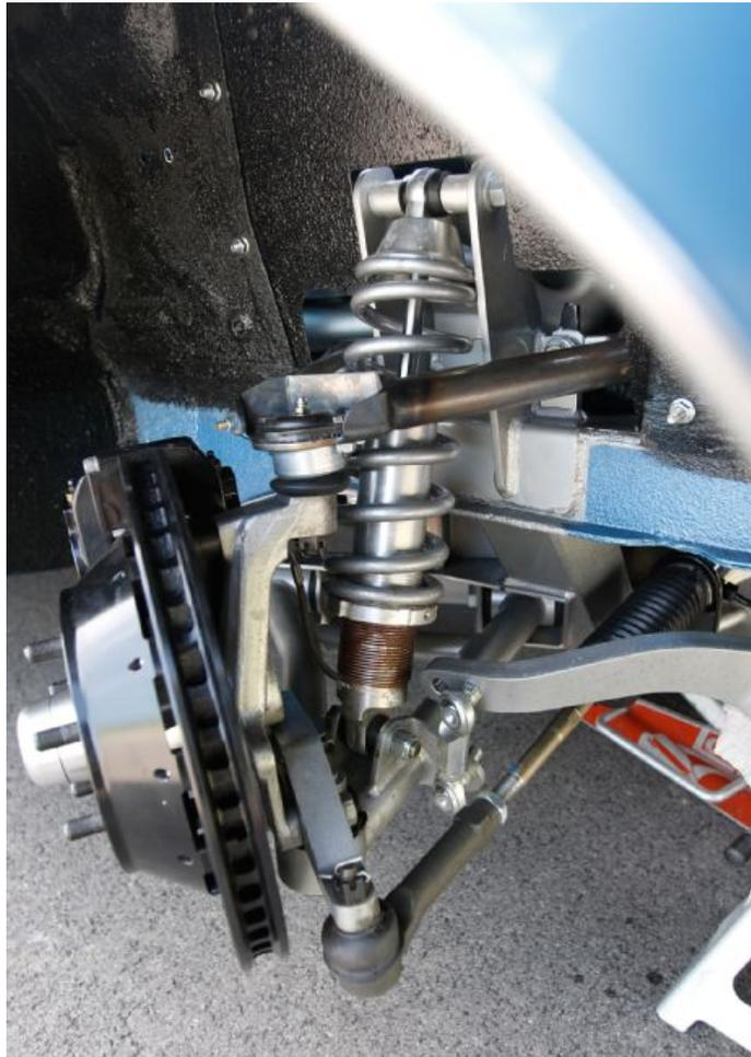
**The heart of this Mustang can be found underneath, with the Heidts Pro-G front and rear suspensions. Up front, the IFS incorporates improved geometry and adjustability for all types of driving.**
