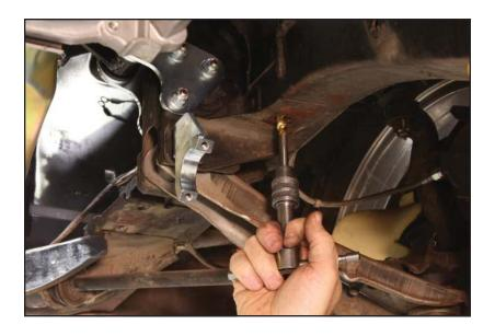
25. On the passenger-side frame rail, loosely bolt the frame bracket to the OEM-crossmember mounting point using the 1/2-13 x 1-1/2" bolt, flat washer, and lockwasher.
