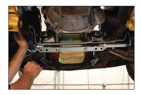
27. On driver-side frame rail, loosely bolt the rack and pinion's attached frame bracket to the OEM-crossmember mounting point, using the same hardware as the passenger side bracket.
