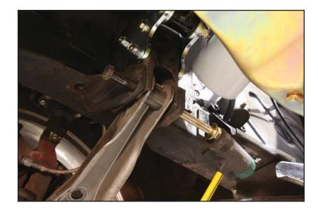
17. With the suspension at full extension, the lower control arms can be safely unbolted. Use caution as the arm may shift once the bolt is removed.
